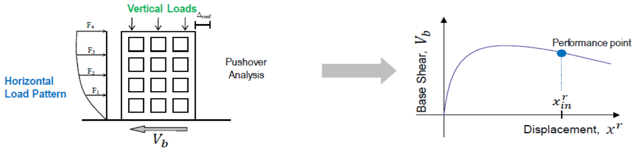
Fig 3.3: Pushover Analysis for Performance Evaluation of Building
