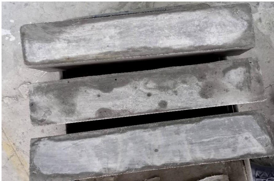
Figure : Beams before corrosion
