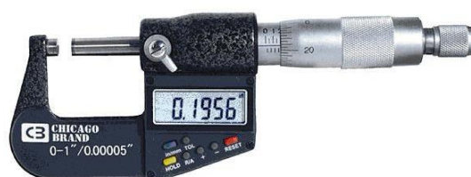
Figure 3.4: Digital Micrometer to measure Dimensional Deviation
