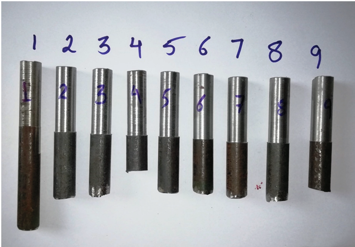
Figure 4.6: EN-9 (heat treated) specimens after machining on CNC turning machine
