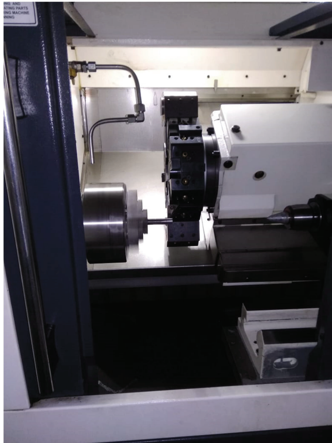
Figure 4.4 Turning of Heat Treated Steel Specimen
