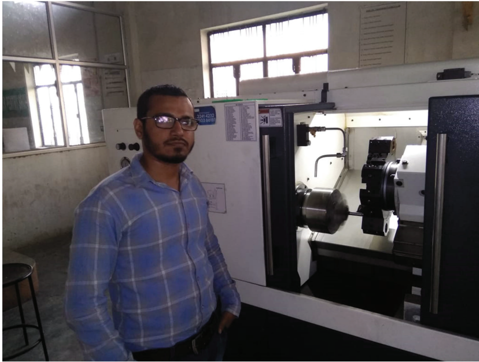
Figure 4.3 ACE CNC Turning Machine with Heat Treated Steel (EN-9) Specimen
