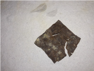
Fig. 4.2 Sample after biodegradation by composting after 3 days
