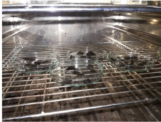
Fig.3.6. Samples kept in oven for moisture content measurement
