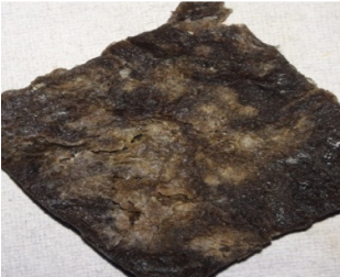
Fig. 4.3. Sample after biodegradation by bench-scale simulated composting after 3 days
