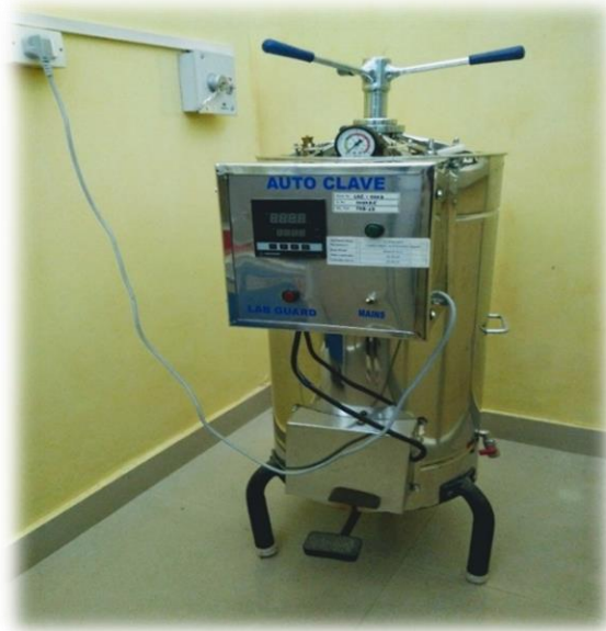
Figure No.16: Autoclave
