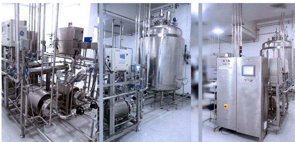
Fig.2. Purified water system
