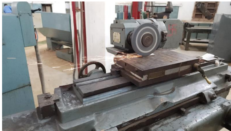
Fig 4.1 Setup for grinding wheel on Tool and cutter grinding wheel
