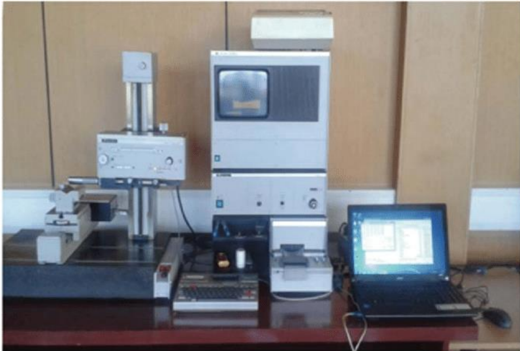
Fig 18: Talysurf setup for measuring surface roughness
