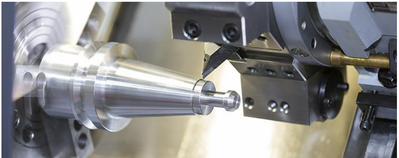
Fig 2: Basic turning operation on Lathe
