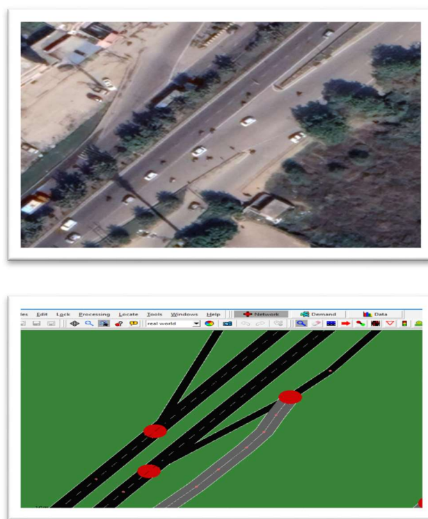
Fig 1. Section for the study and corresponding model in SUMO
