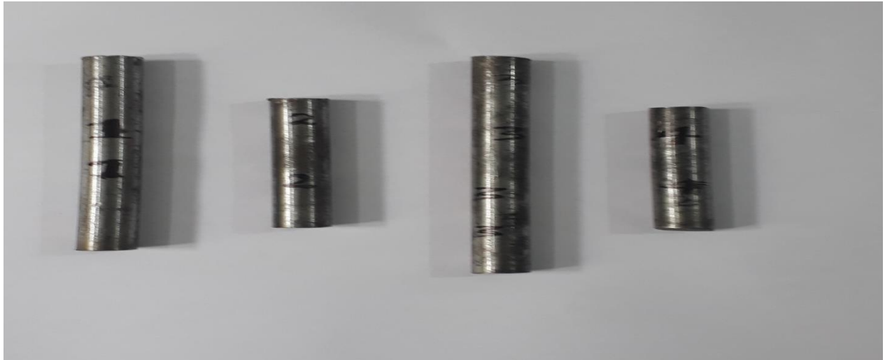
Fig 3.10(a) Test specimen of alloy steel before experiment
