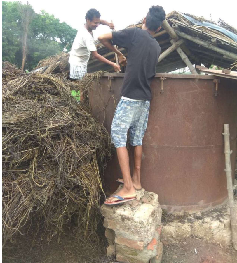
Figure 15: Workers removing processed hay out of boiling vessel
