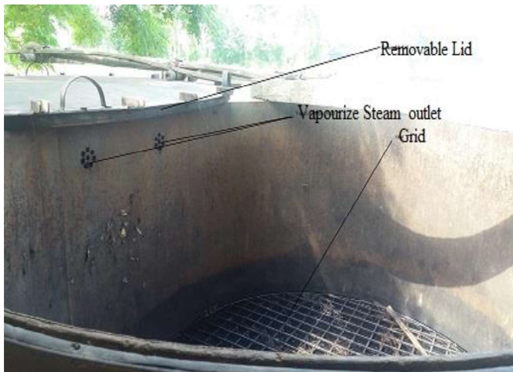
Figure 9: Internal view of Boiler drum
