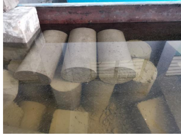
Fig 3.13: Curing of Cylinder
