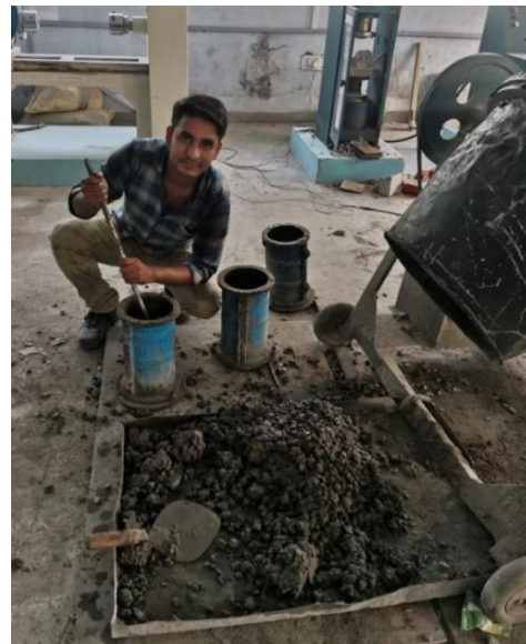
Fig 3.11 : Casting of Cylinder
