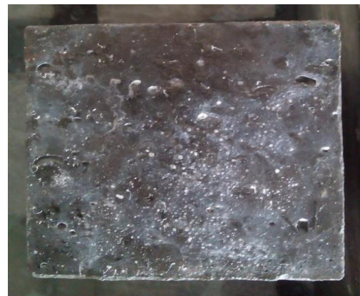
Figure- Pores start filling up by calcium carbonate
