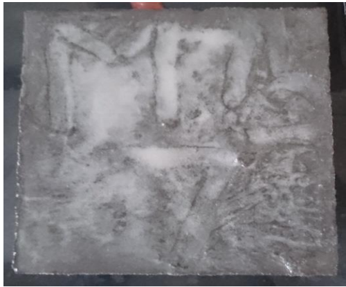
Figure- Calcium carbonate precipitation formed
