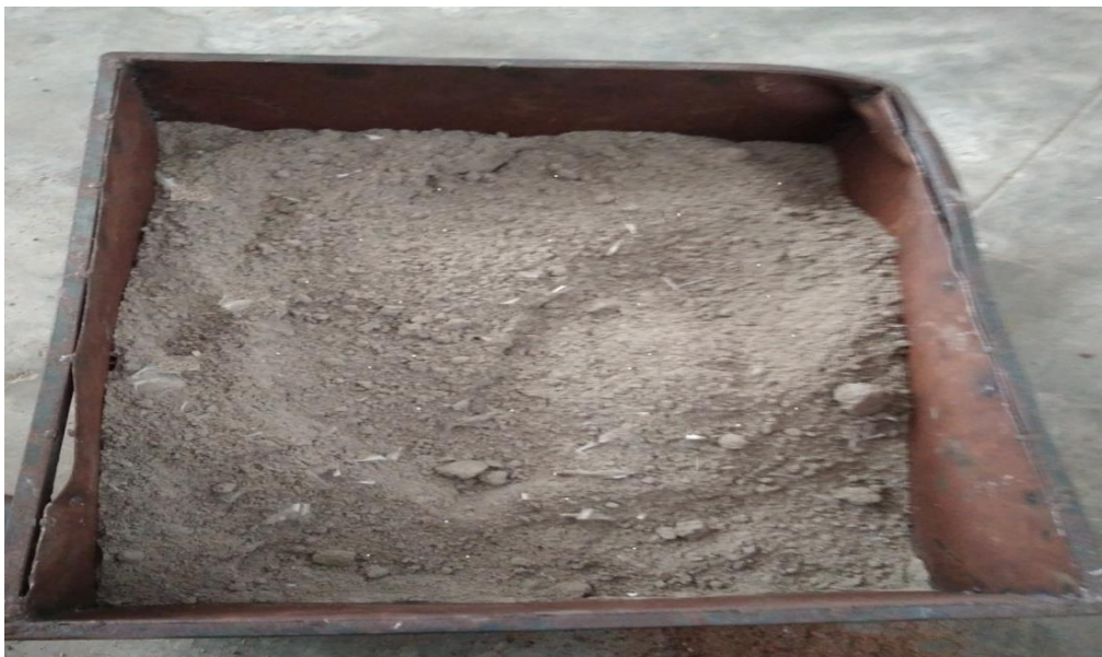
Figure .15 mixture of poly propylene, stone dust and fly ash
