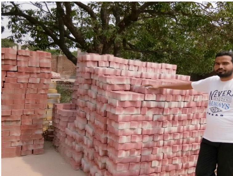
Figure . 4 A Stack of manufactured interlocking concrete block pavers at the factory side
