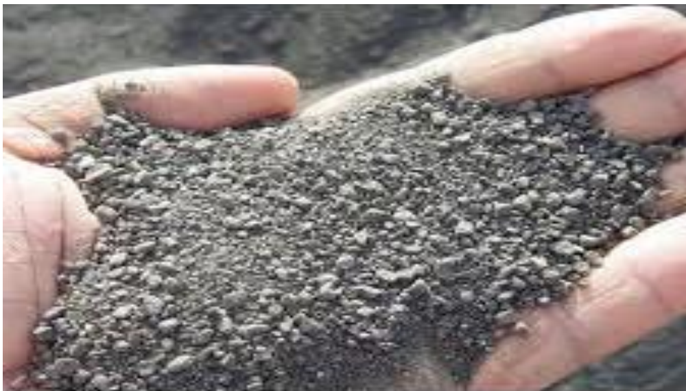
Figure.13 (b) stone dust used in experimental program
