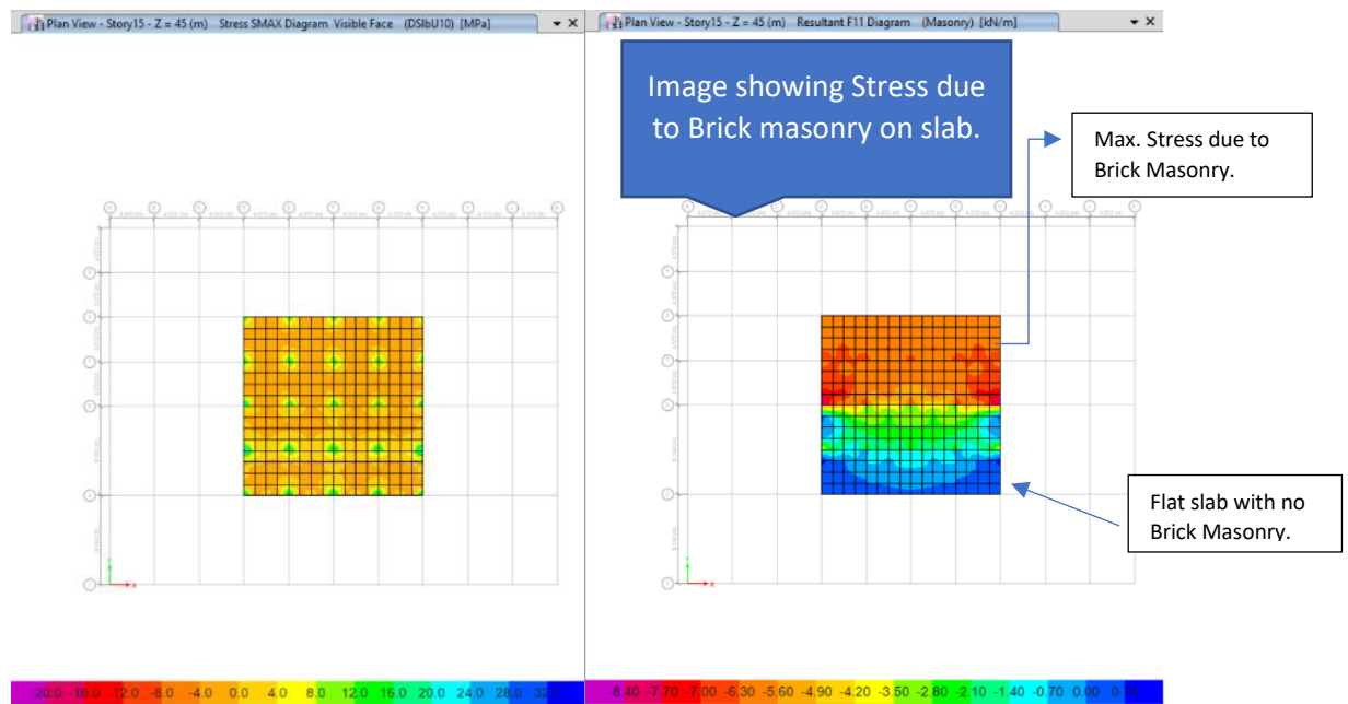
Fig 4.6: Comparison in stress between in the area of flat and waffle slab.
