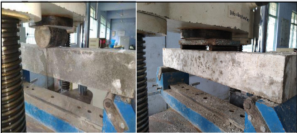
Fig.16 Testing on FTM (At One Point Load and Two Point Load)
