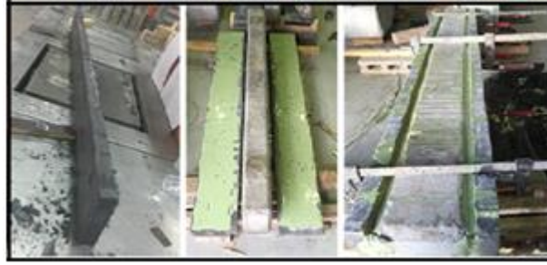
Fig. 4. Strengthened Beams Prefabricate UHPFRC Strips using Epoxy Adhesive Bonding
