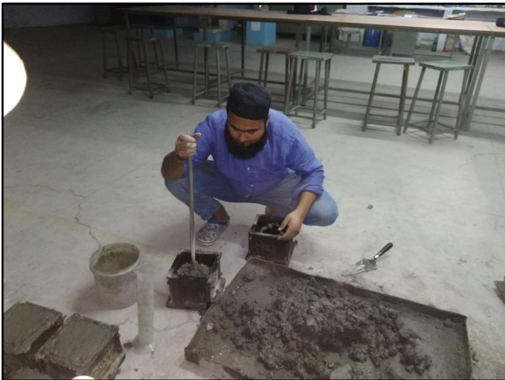
Fig.11 Casting of Cube
