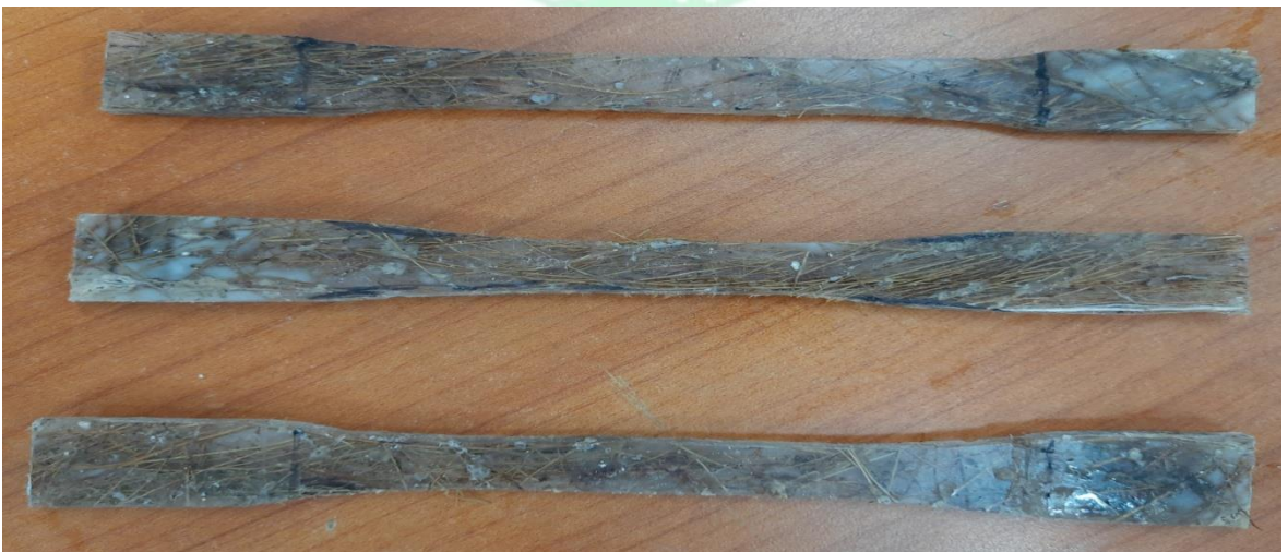
Fig 4.1.1(e)-Tensile specimen before fracture (Batch 4)
