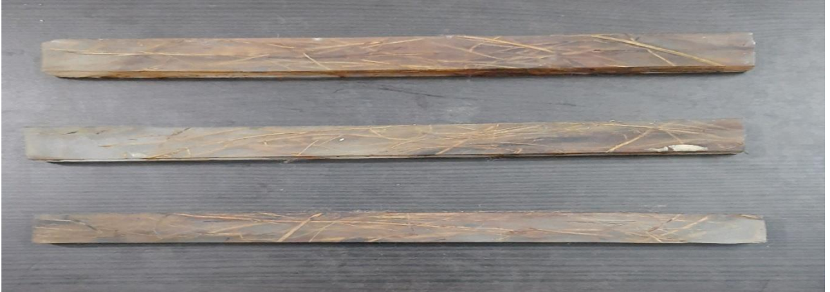
Fig. 4.1.2(c)-Flexural specimen before fracture (Batch3)
