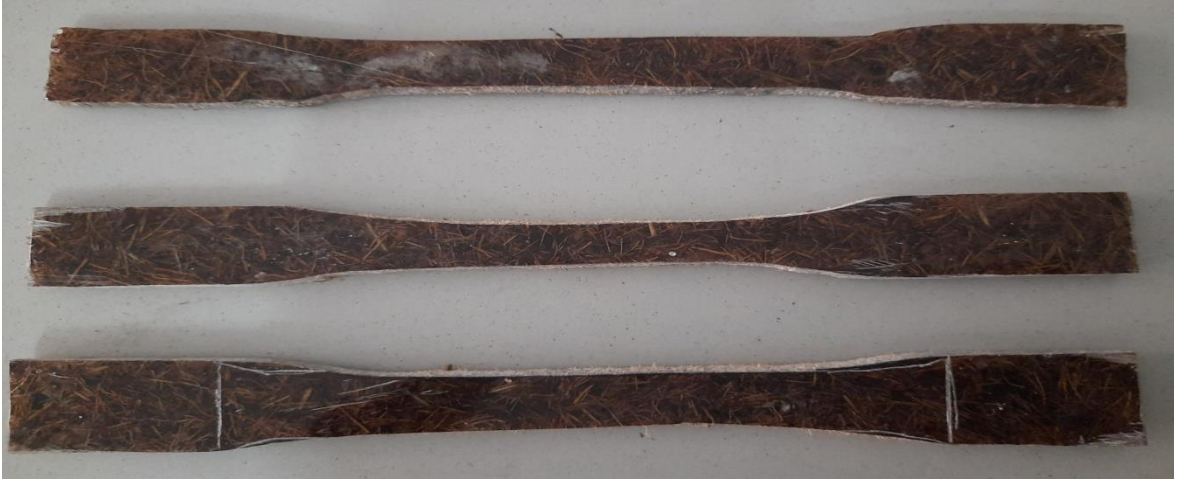
4.1.1(c)- Tensile specimen before fracture (Batch 2)
