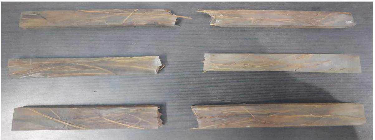
Fig. 4.1.2 (g)-Flexural specimen after fracture (Batch 3)
