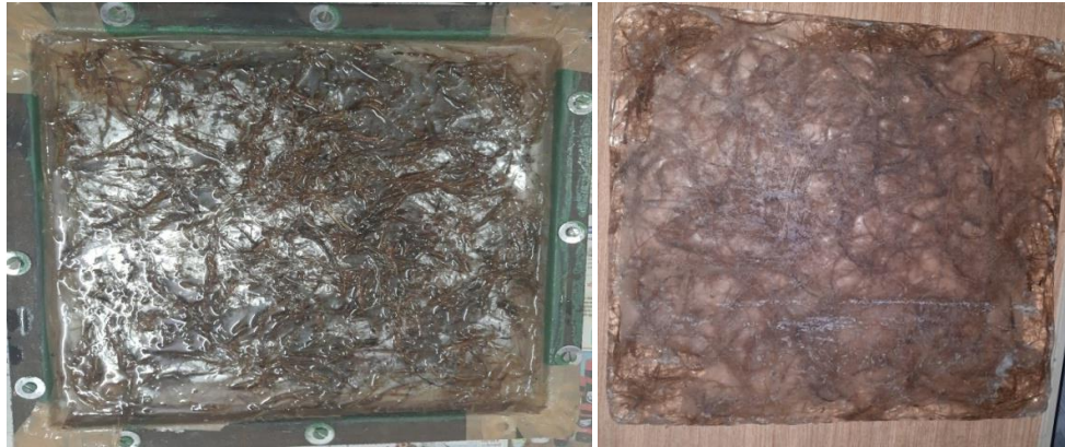
Fig-3.2.2(b) Mould box with treated fibers and resin mixture
