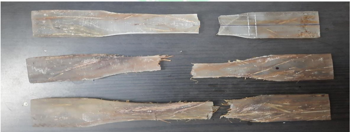
Fig 4.1.1(h)-Tensile specimen after fracture (Batch 3)
