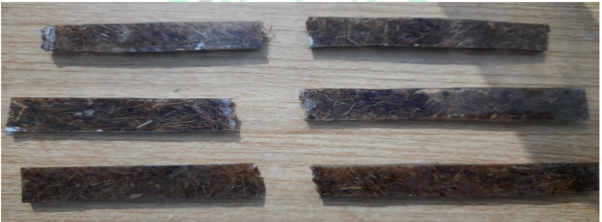
Fig. 4.1.2(e)-Flexural specimen after fracture (batch 1)
