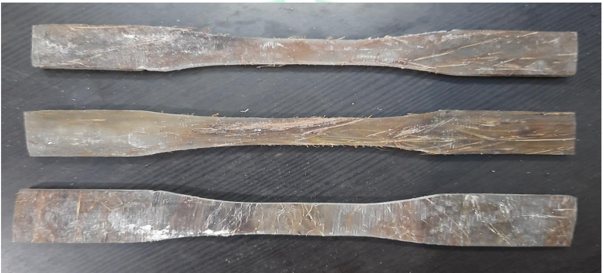
Fig- 4.1.1(d)-Tensile specimen before fracture (Batch 3)
