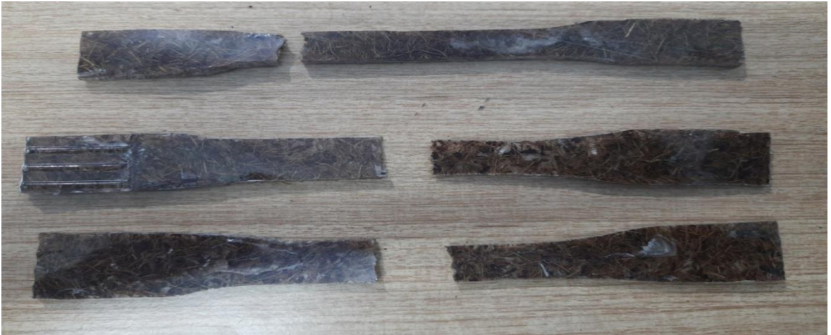
Fig. 4.1.1(f)-Tensile specimen after fracture (Batch 1)
