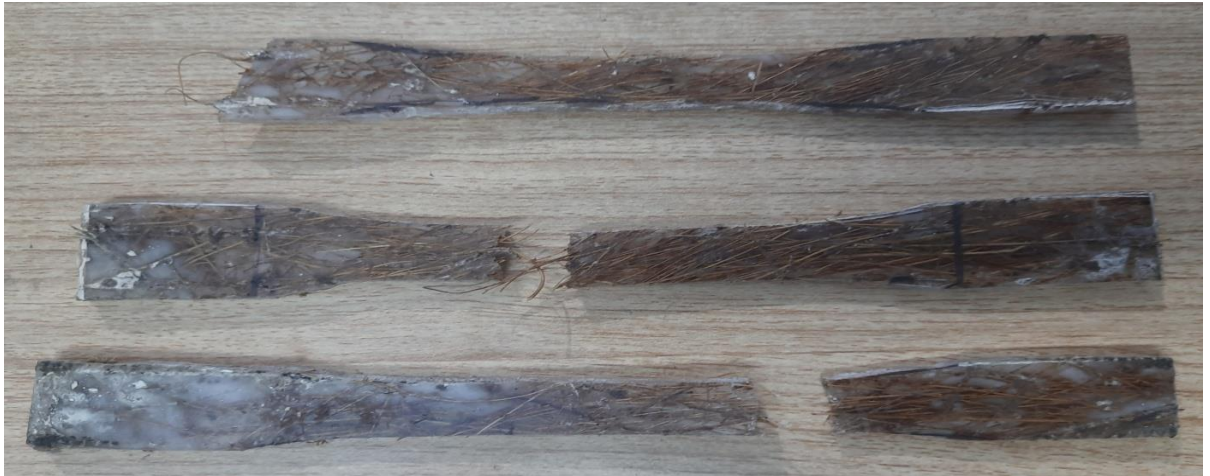
Fig 4.1.1(i)- Tensile specimen after fracture (Batch 4)
