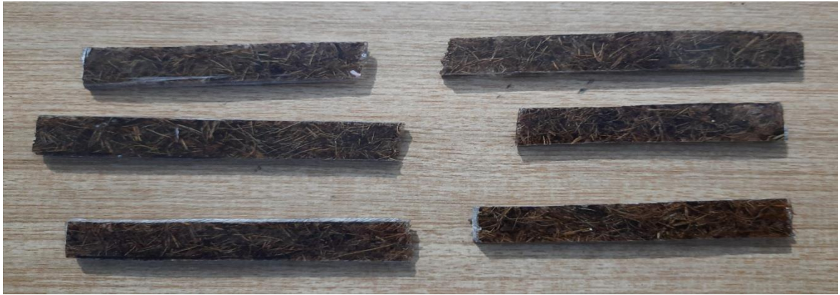
Fig. 4.1.2(f)- Flexural specimen after fracture (batch 2)
