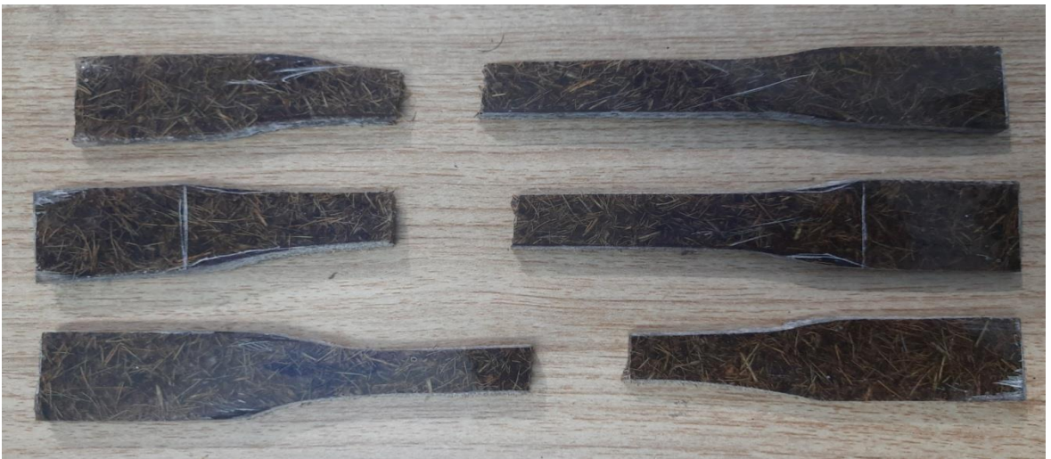
Fig. 4.1.1(g) tensile specimen after fracture (Batch 2)
