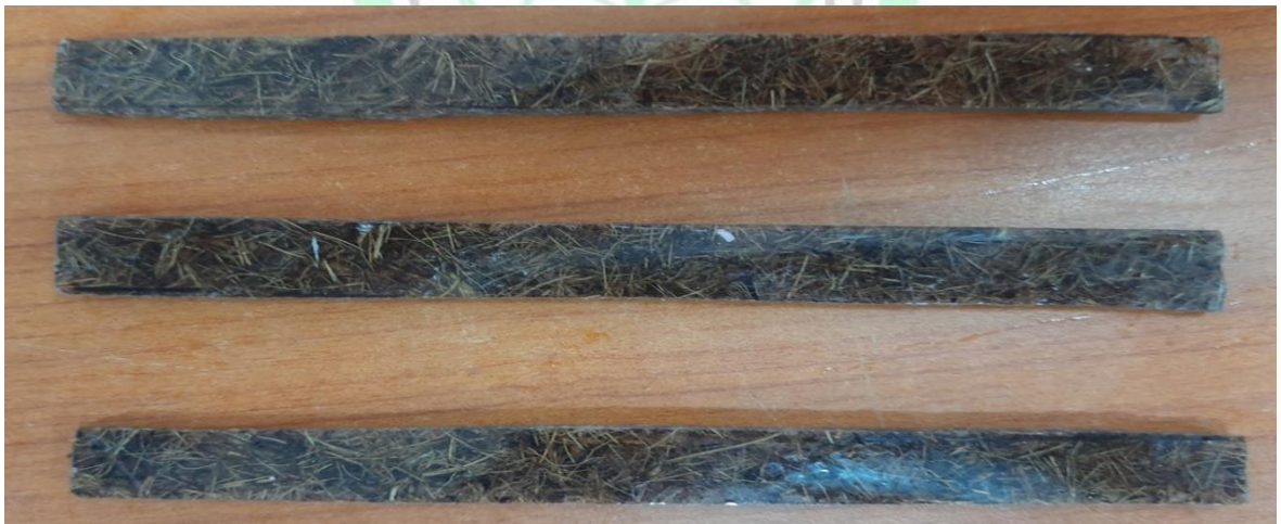
Fig. 4.1.2 (b) Flexural specimen before fracture (Batch 2)
