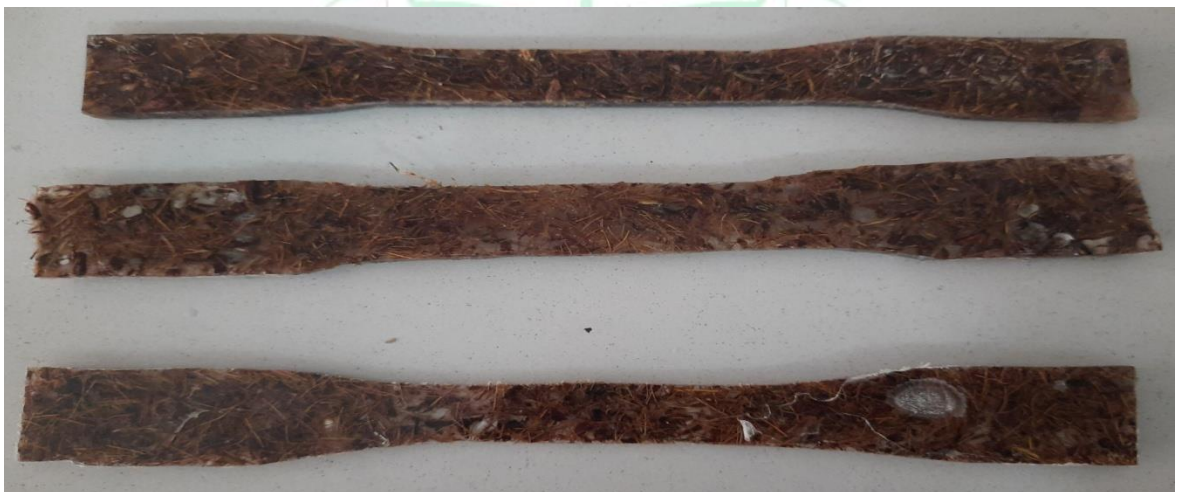
Fig 4.1.1(b) tensile specimen before fracture (Batch 1)
