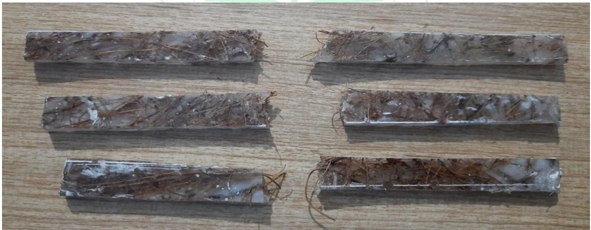
Fig. 4.1.2(h)-Flexural specimen after fracture (batch 4)
