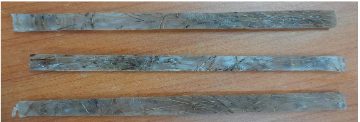
Fig. 4.1.2(d) Flexural specimen before fracture (Batch 4)
