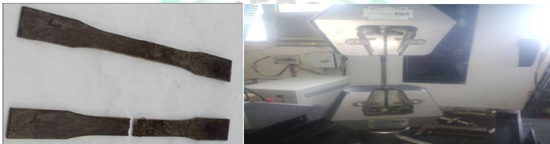
Fig. 4.23. Tensile Test Specimen Before and After Testing.
