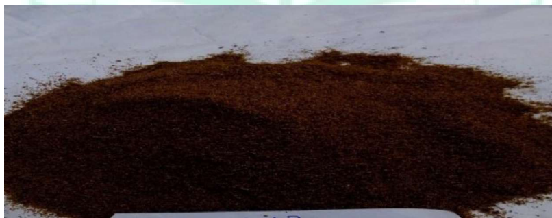
Fig. 4.6. Wood Powder Fiber 740 \mu\text{m} Size.
