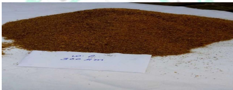
Fig. 4.5. Wood Powder, Fiber 300 \mu\text{m} Size.
