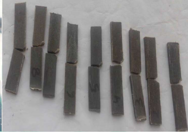
Fig. 4.29. Impact Sample after Testing.
