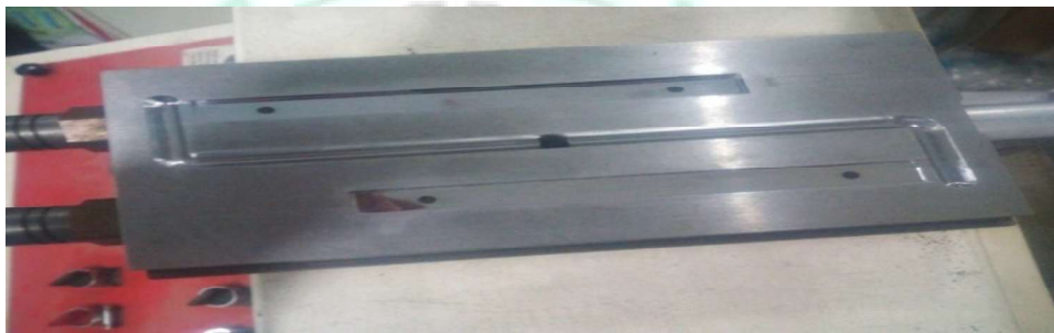
Fig. 4.19. Flexural Insert Mould.
