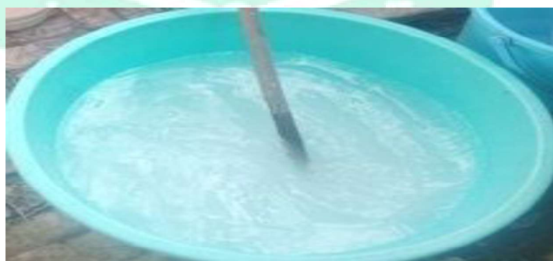
Fig. 4.10. Preparation of NaOH Pellets Solution.
