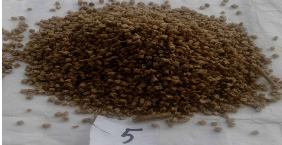
Fig. 4.16 Compounding Material pellets after Cutting by the Cutter.
