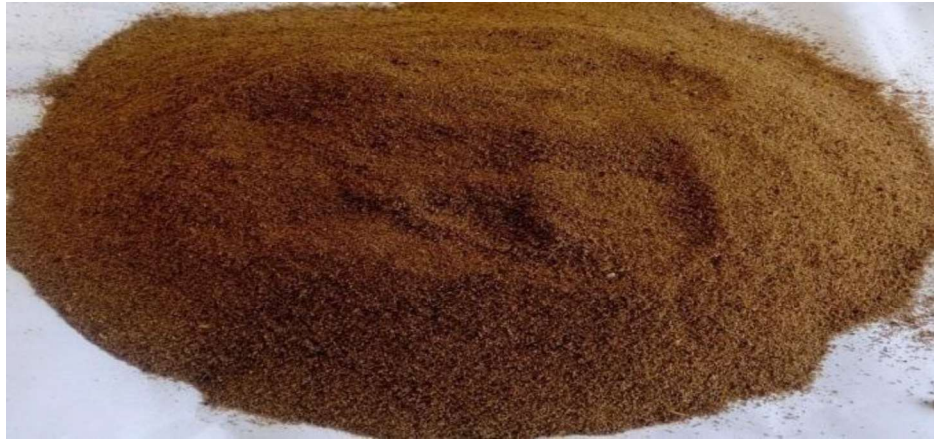
Fig. 4.12. Oven Dried Wood Powder after Treatment.
