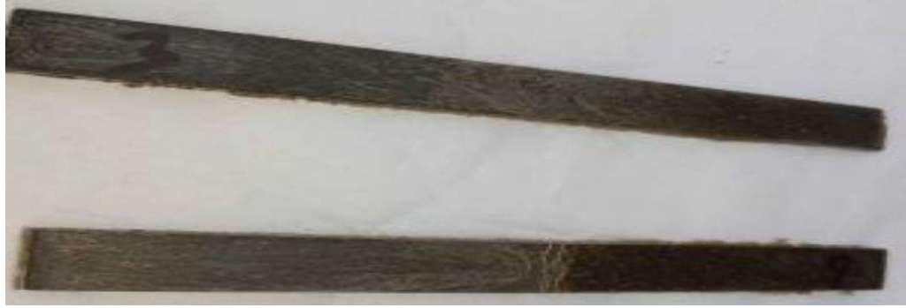
Fig 4.25. Flexural Sample before Testing and After Testing
