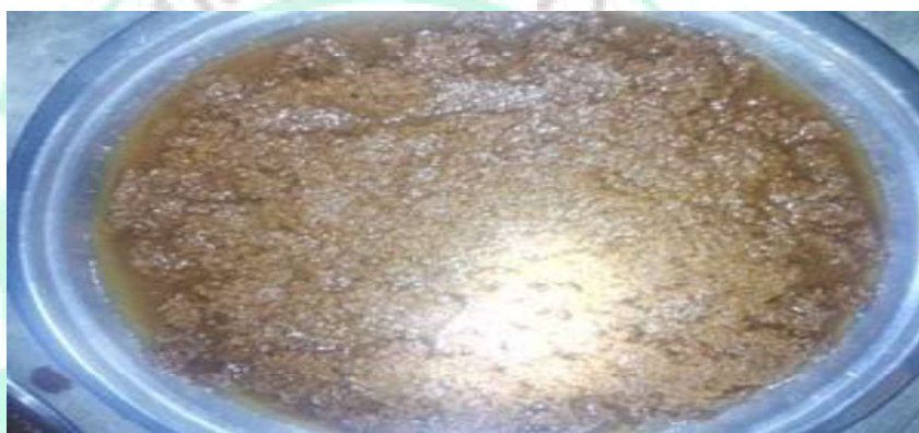
Fig. 4.11. Wood Powder Immersed in NaOH Pellets Solution.
