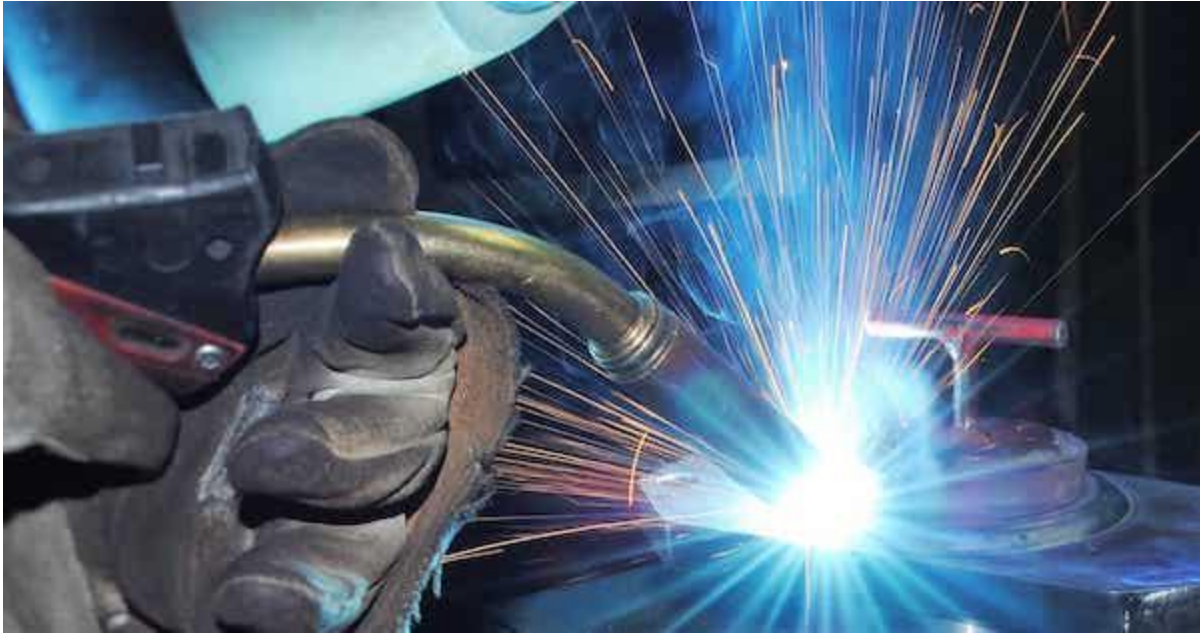
Figure 1.6 Shielding Is Obtained From an Externally Supplied Gas or Gas Mixture
