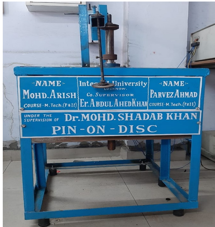
Fig. 1.9 Pin on disc setup
