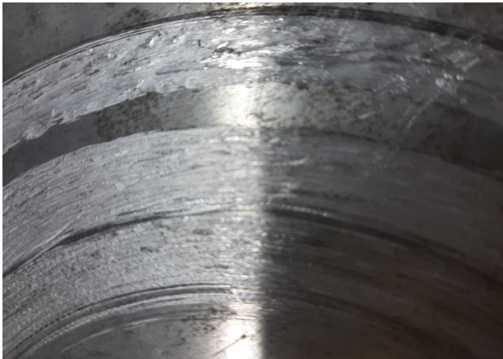
Fig. 2.1 (c) Alumunium5652 alloy disc after test
