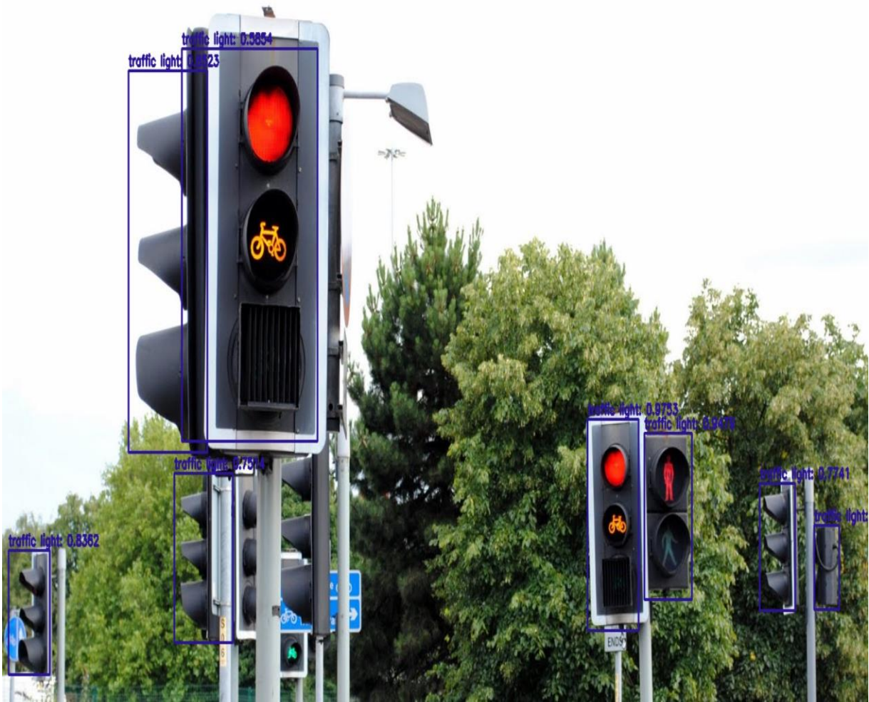
Figure 3: Traffic Signal detection [32]
