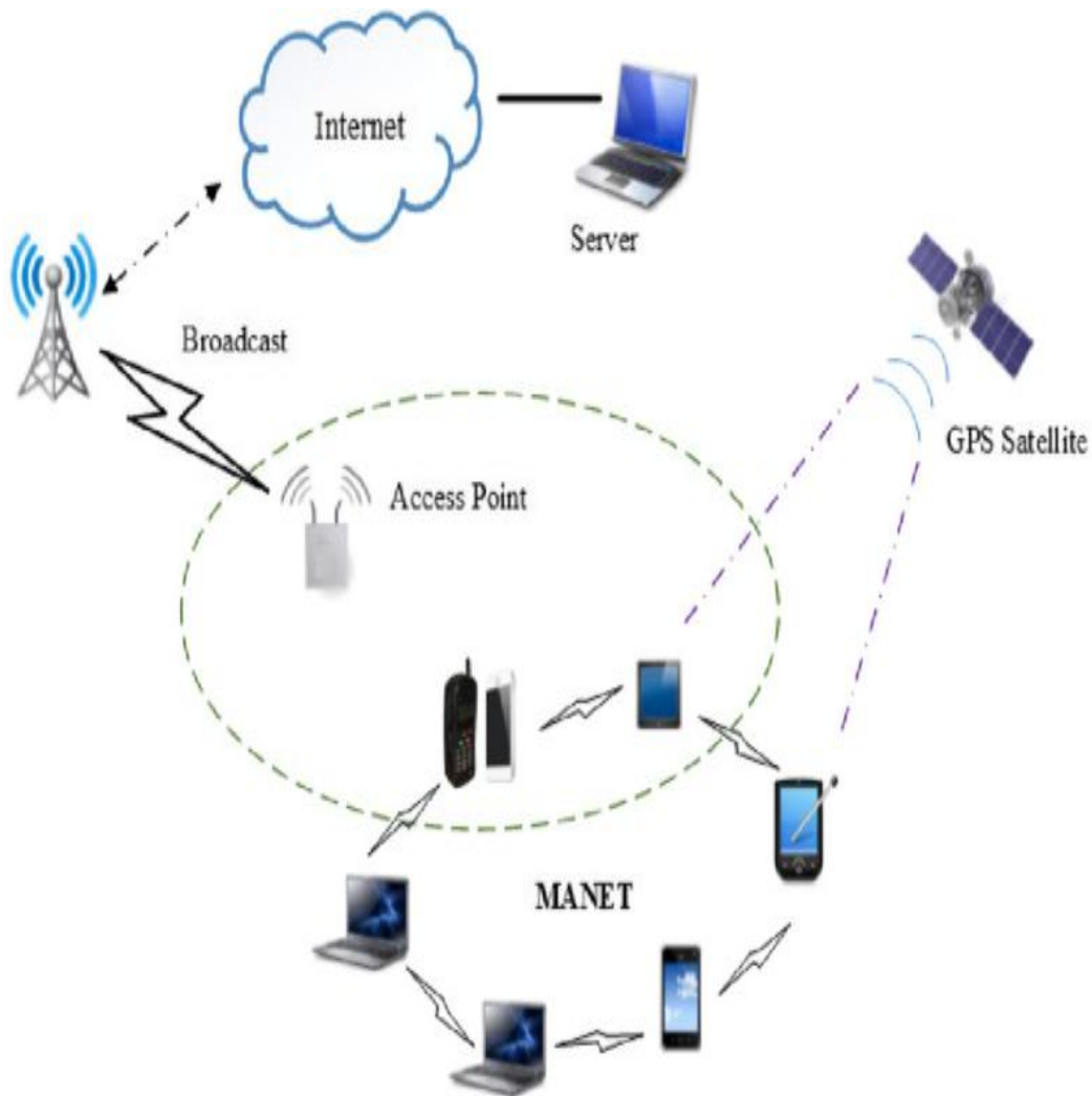
Fig.1.1 Architecture of Mobile ad-hoc Network (MANET)
