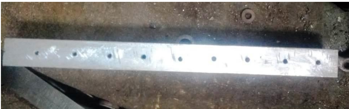
Figure 4.5: Workpiece Bars of Aluminium 6061 after machining
