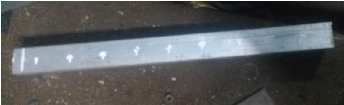
Figure 4.4: Workpiece Bars of Aluminium 6061 before machining
