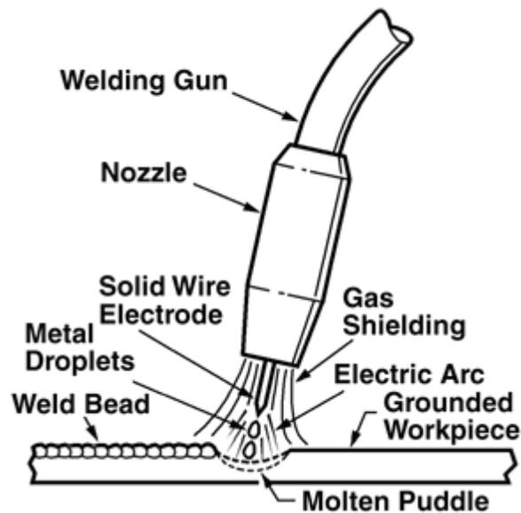
Figure 1.1 MIG Welding Process
