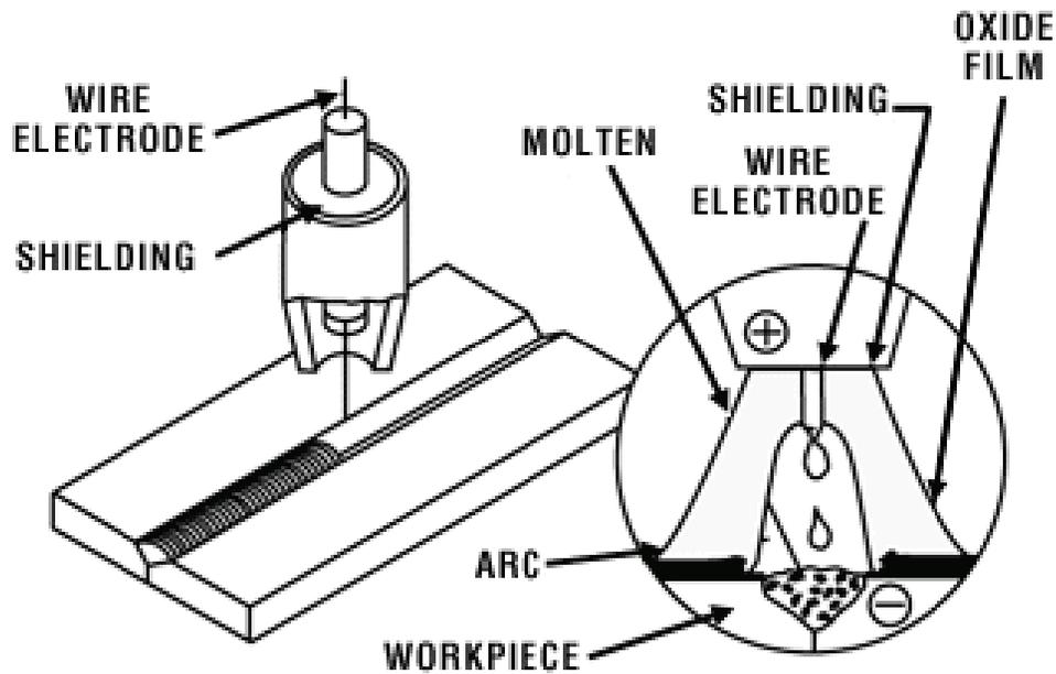
**Figure 1.2 MIG welding area enlarged**
