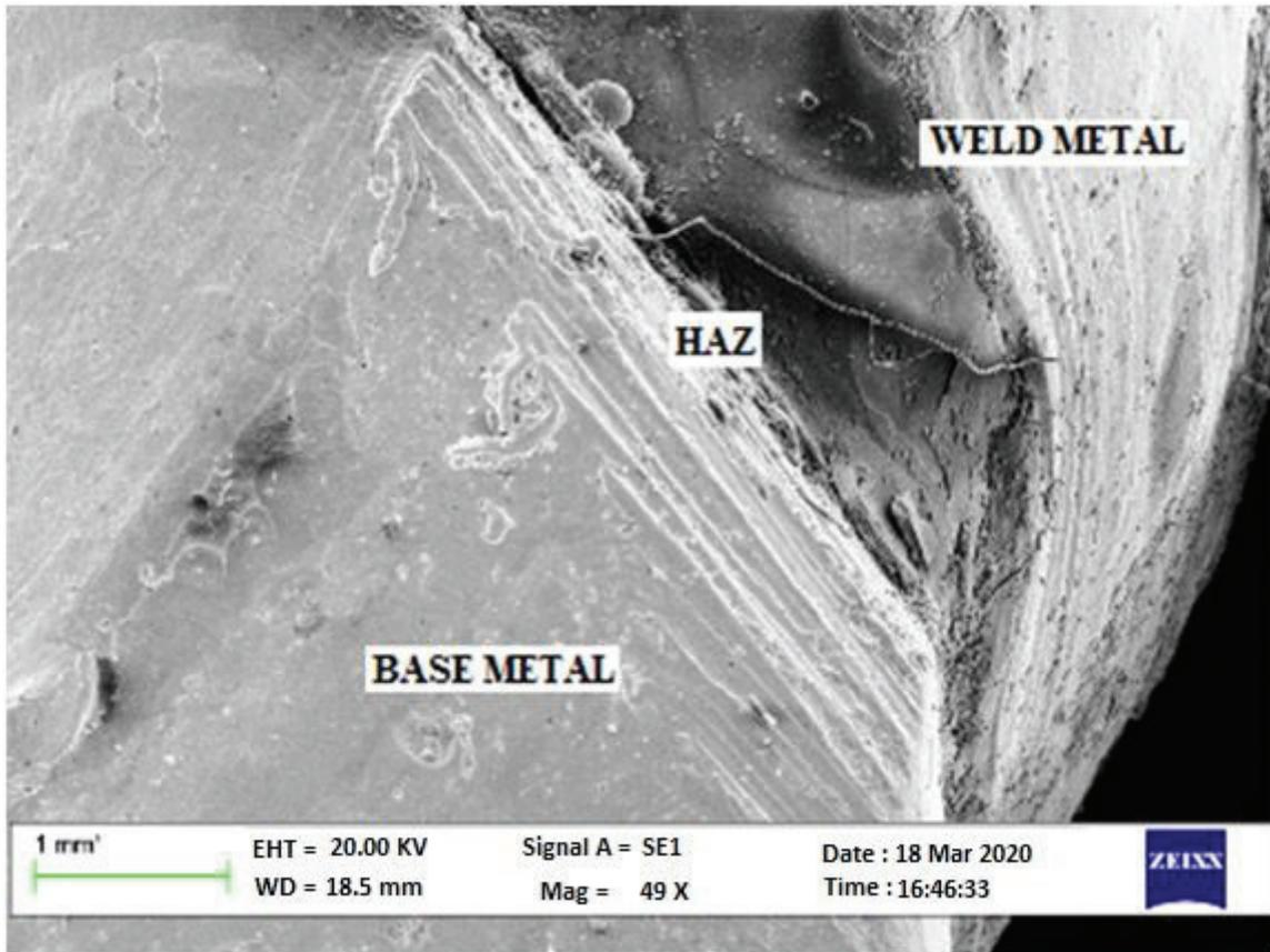
**Figure 5.4 SEM image of sample 3**
