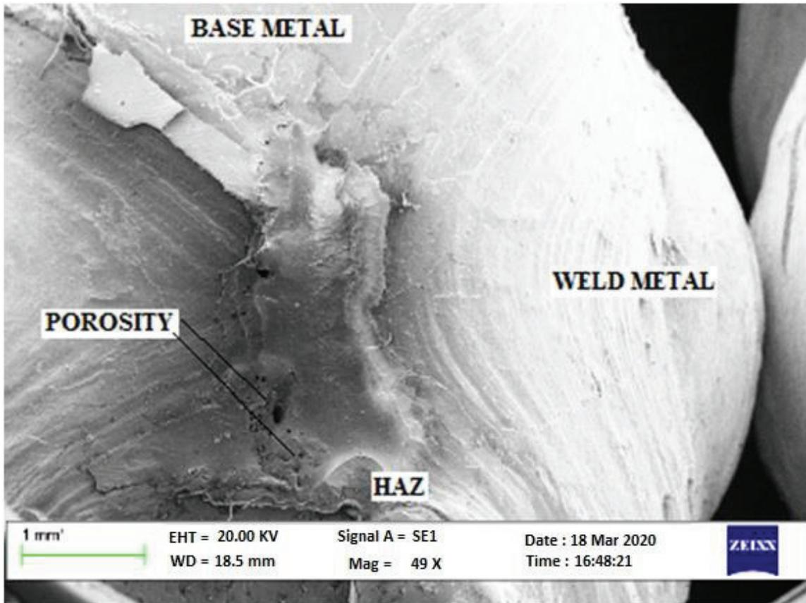
**Figure 5.6 SEM image of sample 7**
