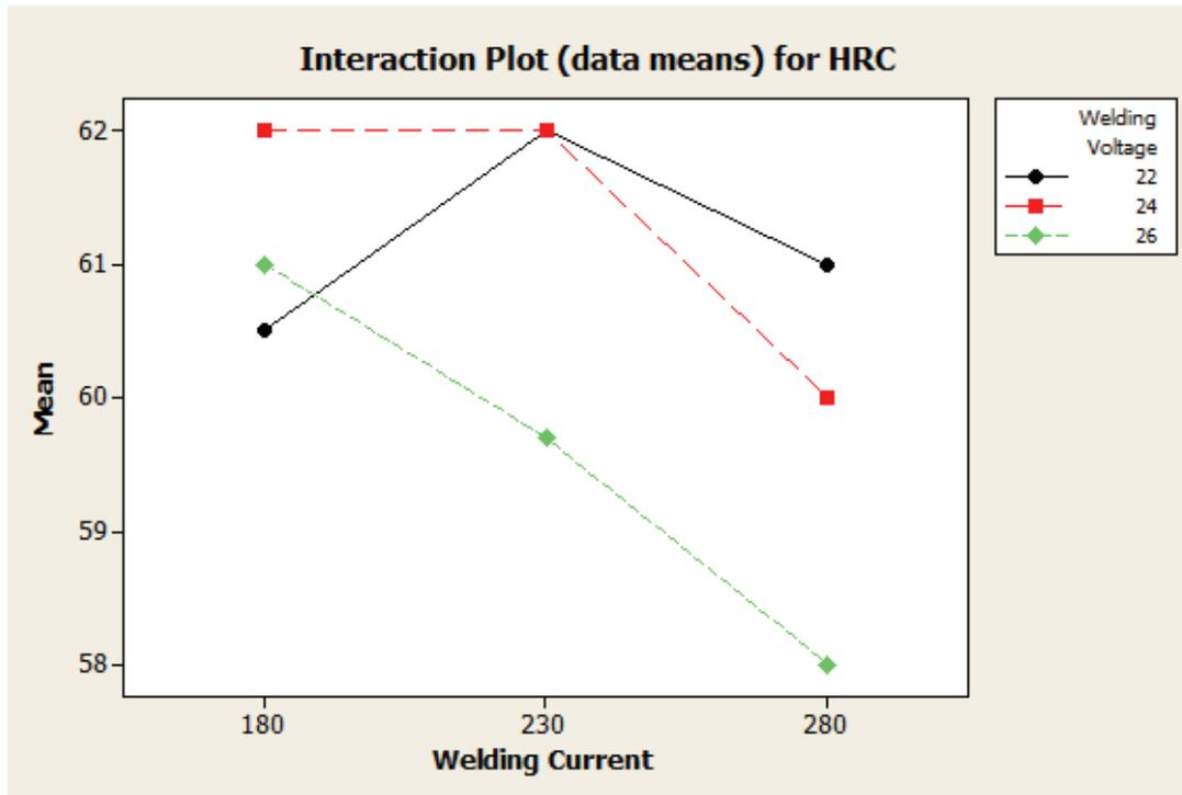
**Figure 5.2: Interaction plot for parameters and Hardness**
