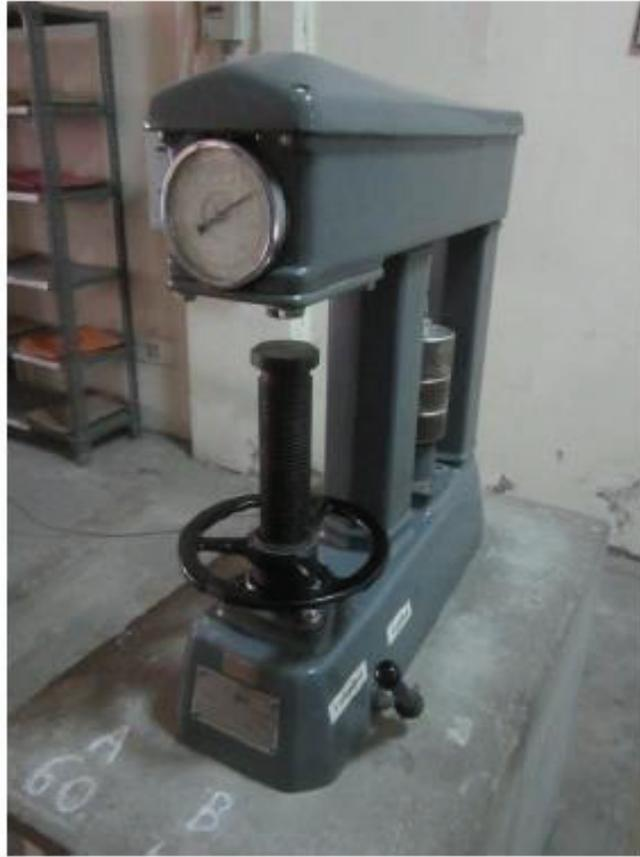
**Figure 4.6 Rockwell Hardness Tester for measuring specimen hardness**
