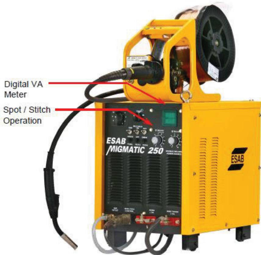
**Figure 4.1: ESAB MIGMATIC 250 MIG welding machine**
