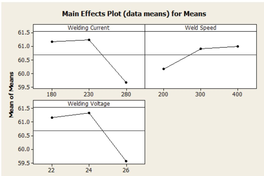
**Figure 5.1: Main effect plot for Hardness**
