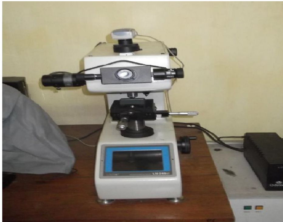
Figure 3.6 Experimental set up for hardness test
