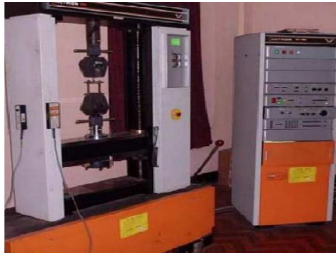
Figure 3.3 Experimental set up for tensile test.
