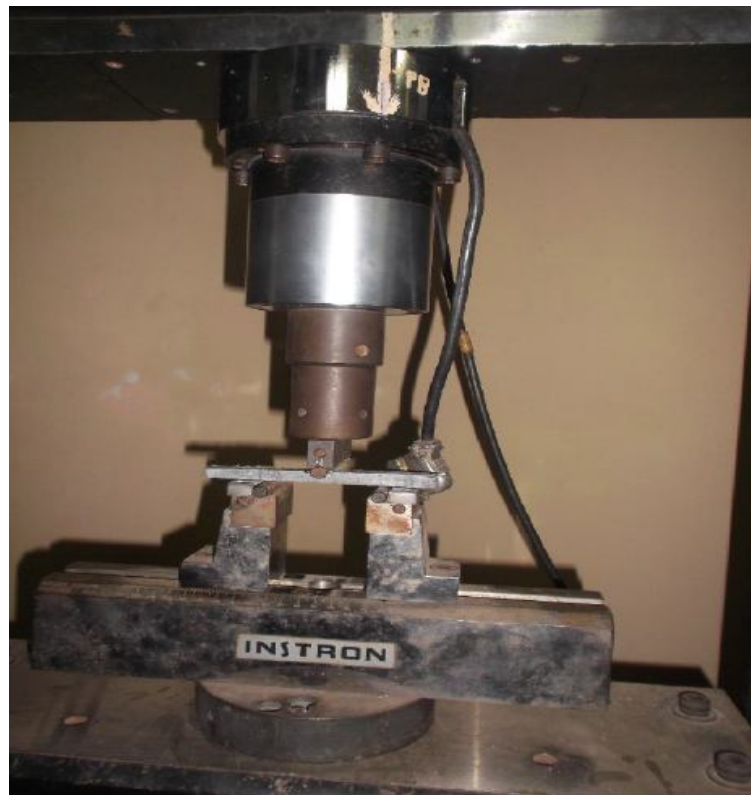
Figure 3.4 Three point bend test loading arrangement.
