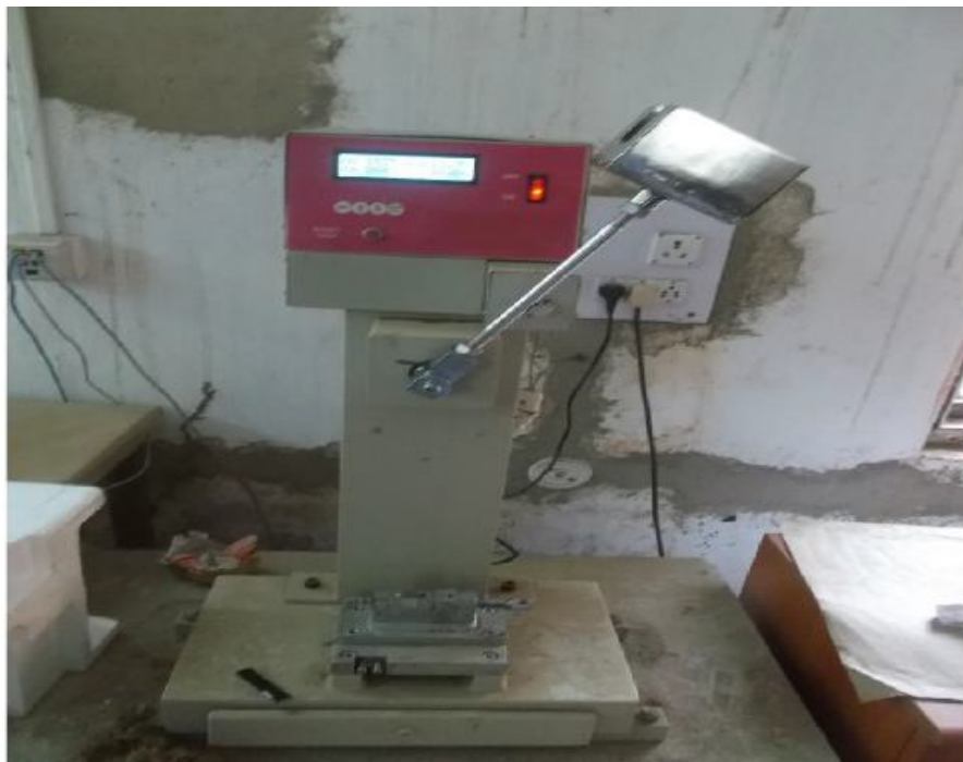
Figure 3.5 Experimental set up for Impact strength
