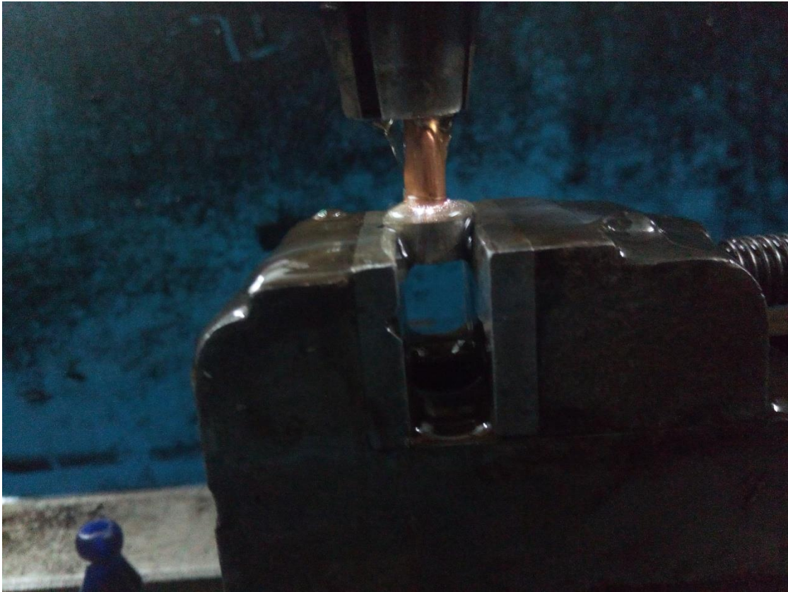
Figure 4.2 Sparking during low level of EDM parameters
