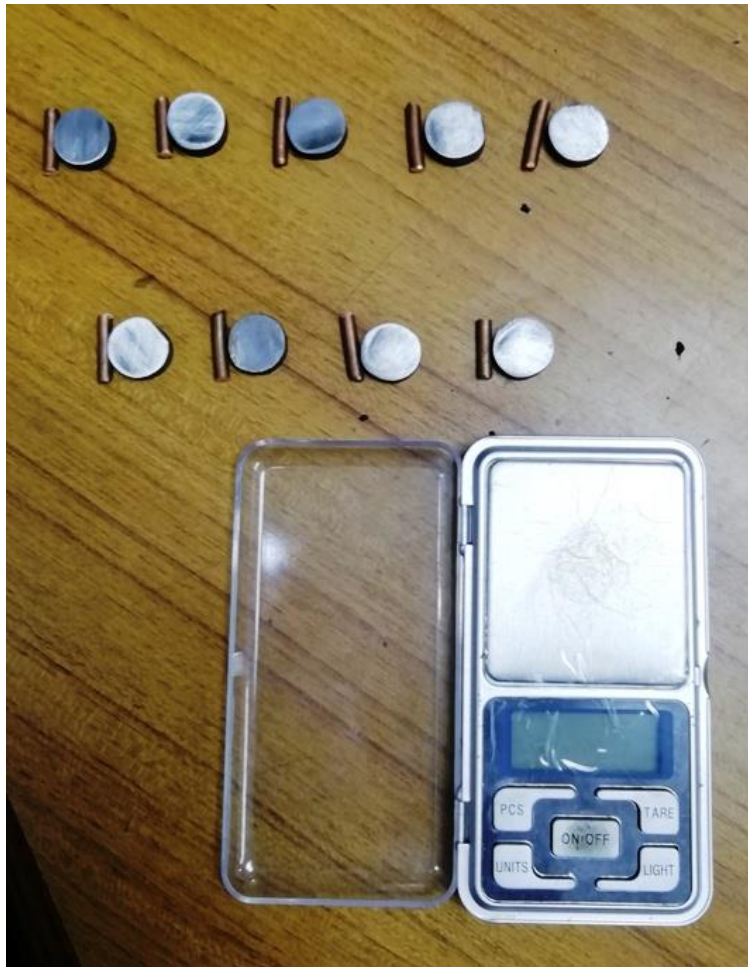
Figure 4.8 Tool and workpiece with digital weighing instrument before machining
