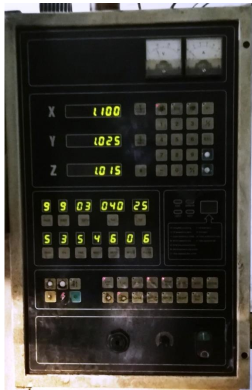
Figure 4.3 Control Panel of EDM Machine
