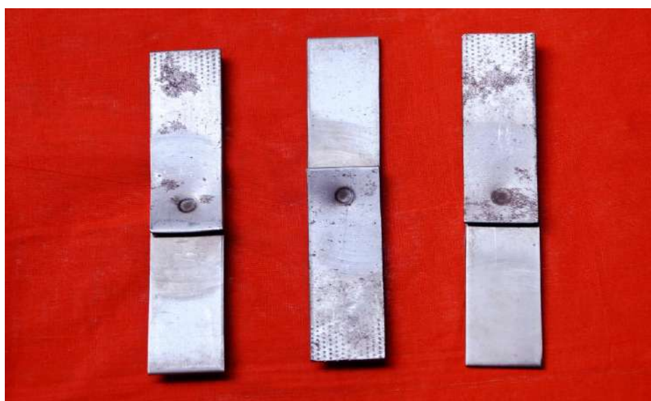
Figure 7.1 Photographic view of TSFL test samples of AIS5052 Similar joints before testing
