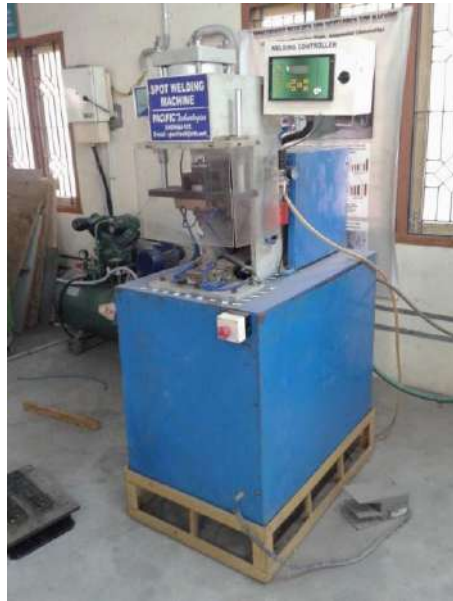
Figure 4.1 Photographic View of the ERSW machine deployed in this study
