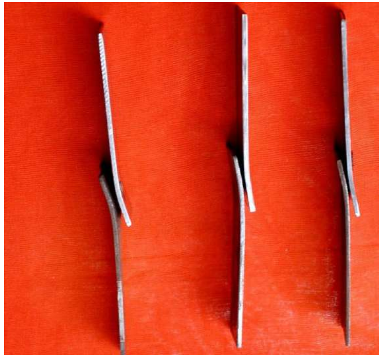
Figure 7.10 Photographic image of TSFL tested samples of AISI1020 – AISI1020 similar welded joints after testing.
