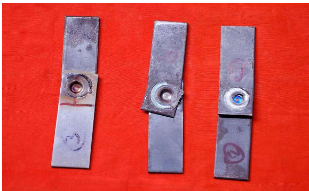
Figure 7.9 Photographic view of TSFL test samples of AISI1020 Similar joints before testing.
