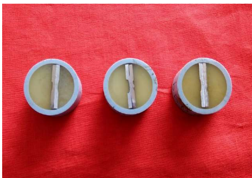
Figure 7.4 (a) Photographic view of microhardness samples of AIS5052 similar joints
