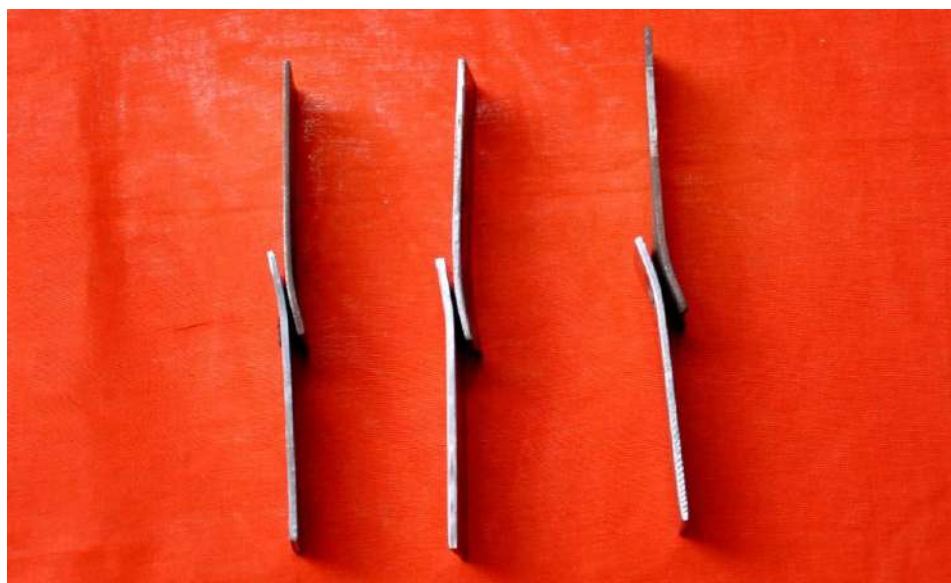
Figure 7.2 Photographic image of TSFL tested samples of AIS5052 – AIS5052 similar welded joints after testing.
