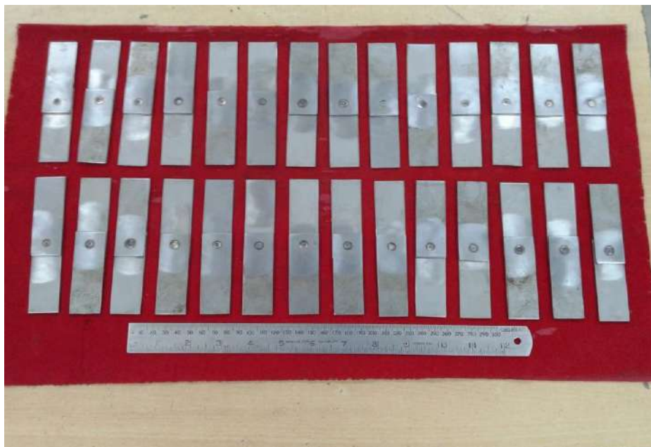
Figure 5.8 Photographic view of the AISI1020-AA1008 samples after the weld
