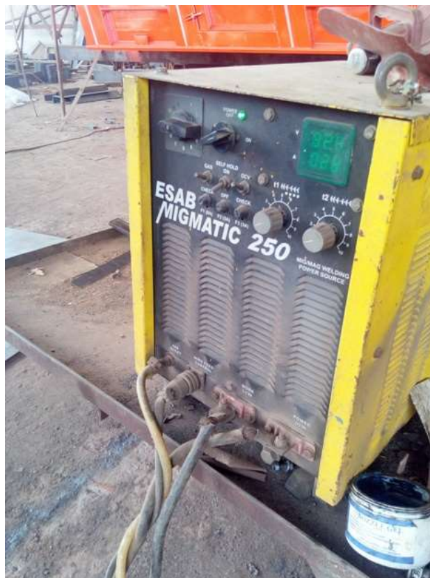
Figure 4.3 MIGMATIC 250 machine panel showing parameters
