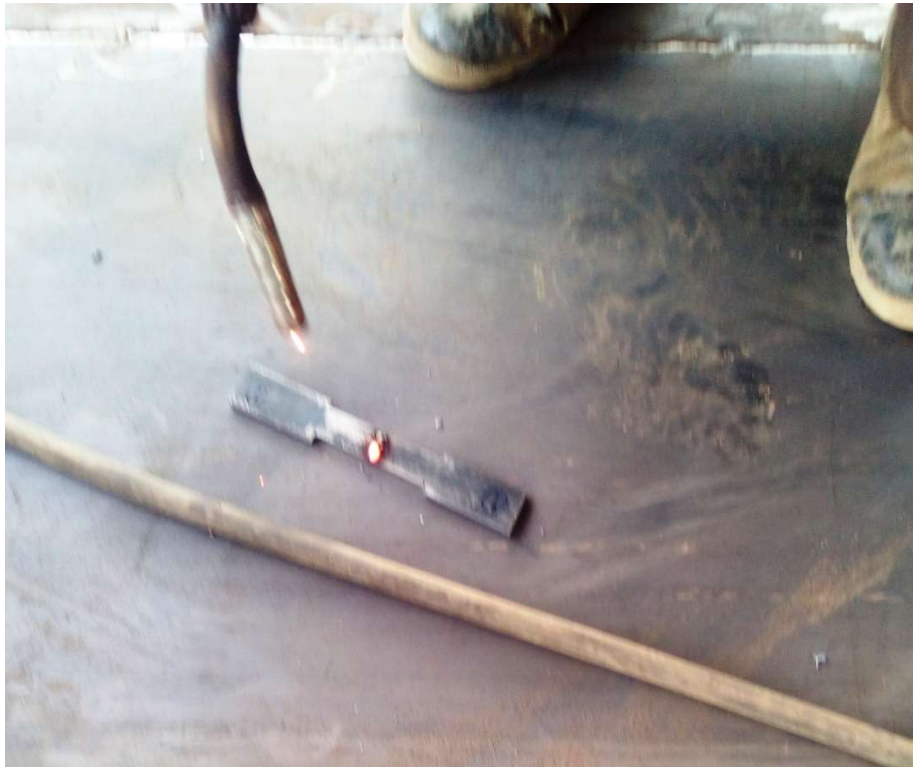
Figure 4.2: Welding of specimens on MIGMATIC 250 machine
