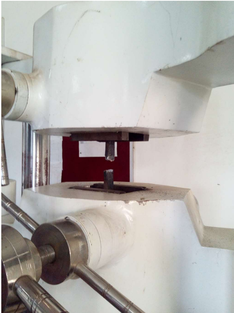
Figure 4.10 Specimen after breaking on UTM machine
