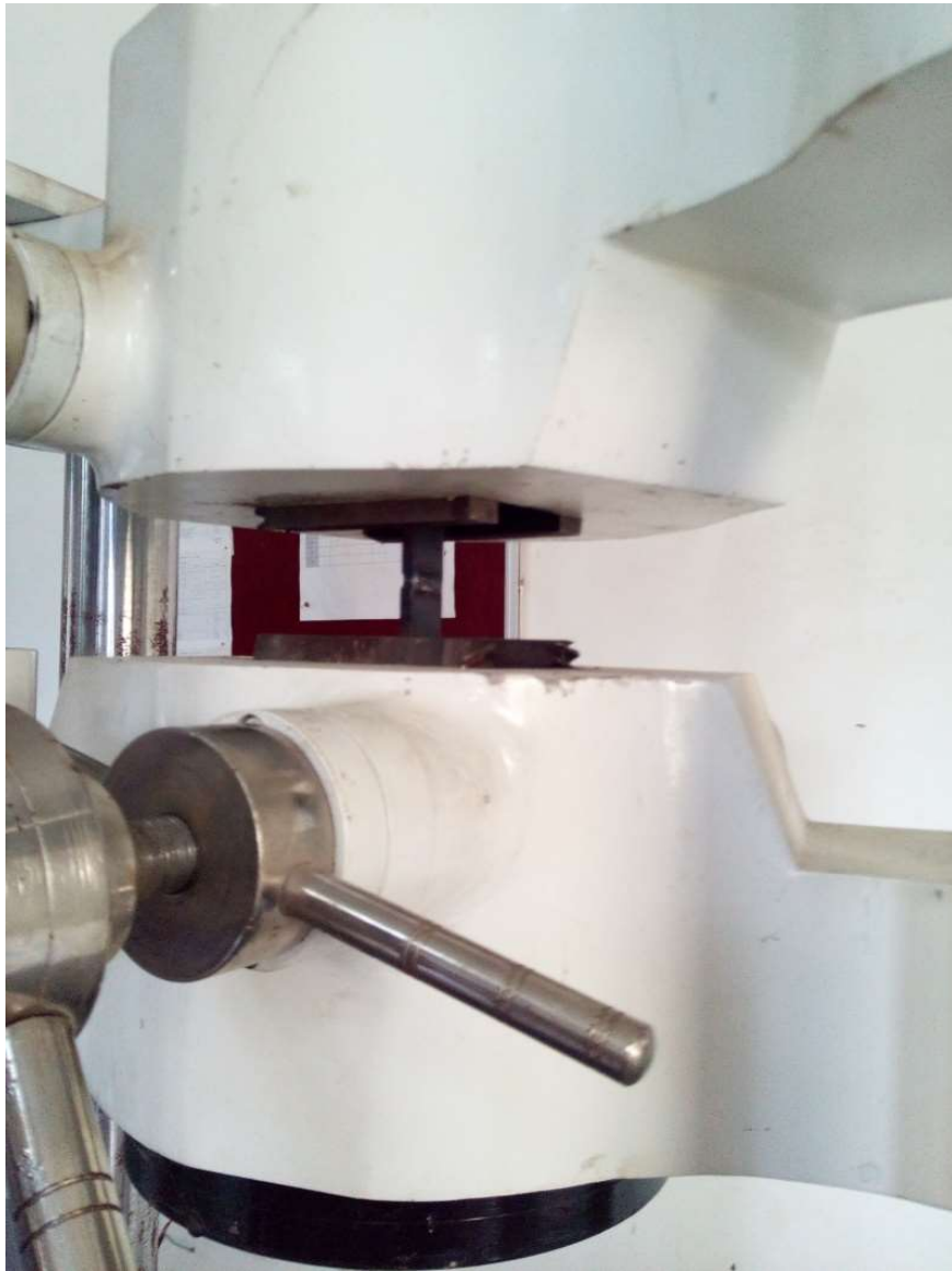
Figure 4.9 Specimen before tensile loading on UTM
