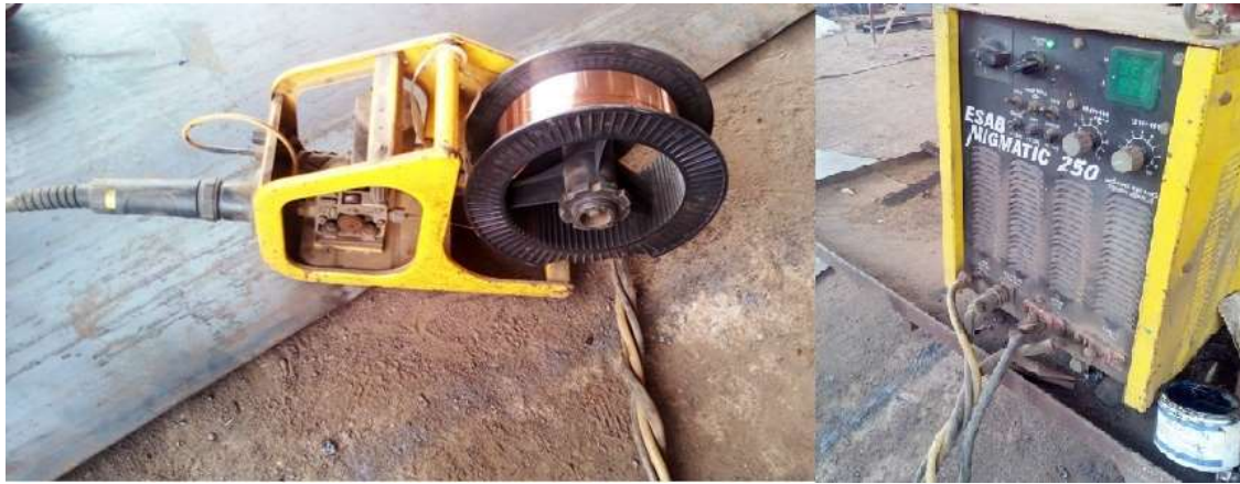
Figure 1.3 Setup of MIG welding for the experiments
