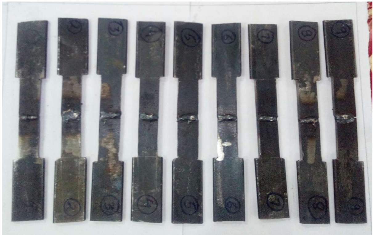
Figure 4.4: Mild Steel welded work pieces
