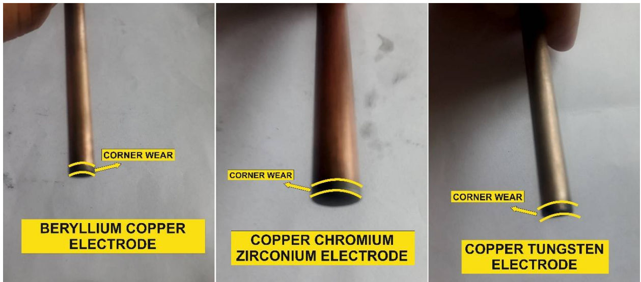
Fig. 5.4 Corner Electrode wear
