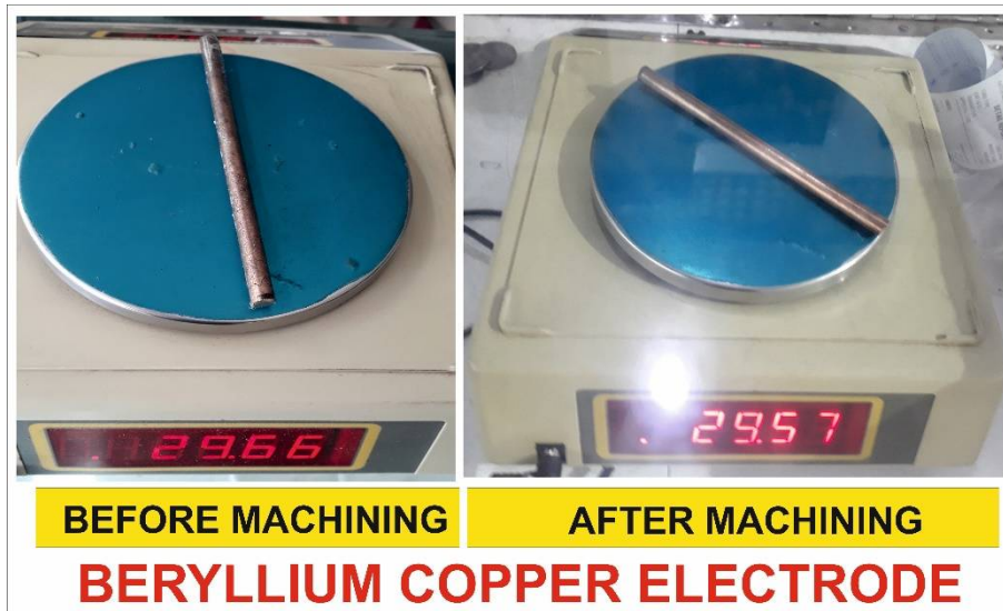
Fig. 4.9.2B Electrode wear of Beryllium copper electrode
