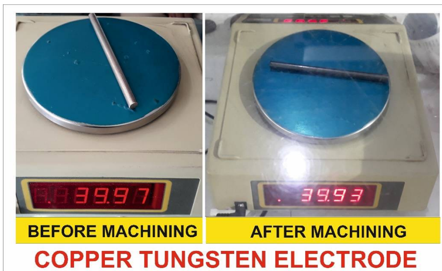
Fig. 4.9.2C Electrode wear of copper Tungsten electrode
