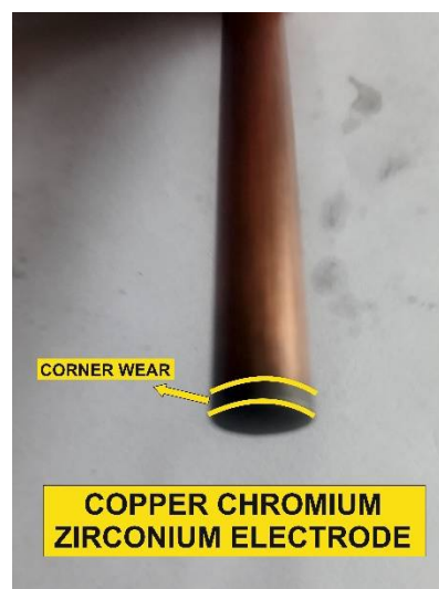
Fig. 5.6 Corner Electrode wear in copper chromium zirconium
