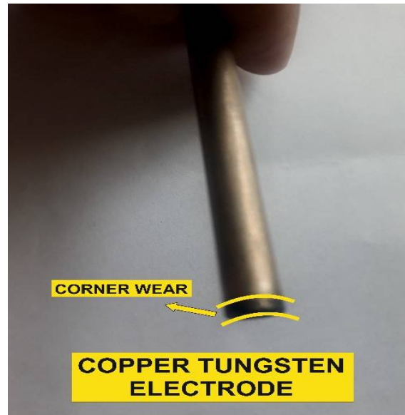
Fig. 5.5 Corner Electrode wear in copper tungsten
