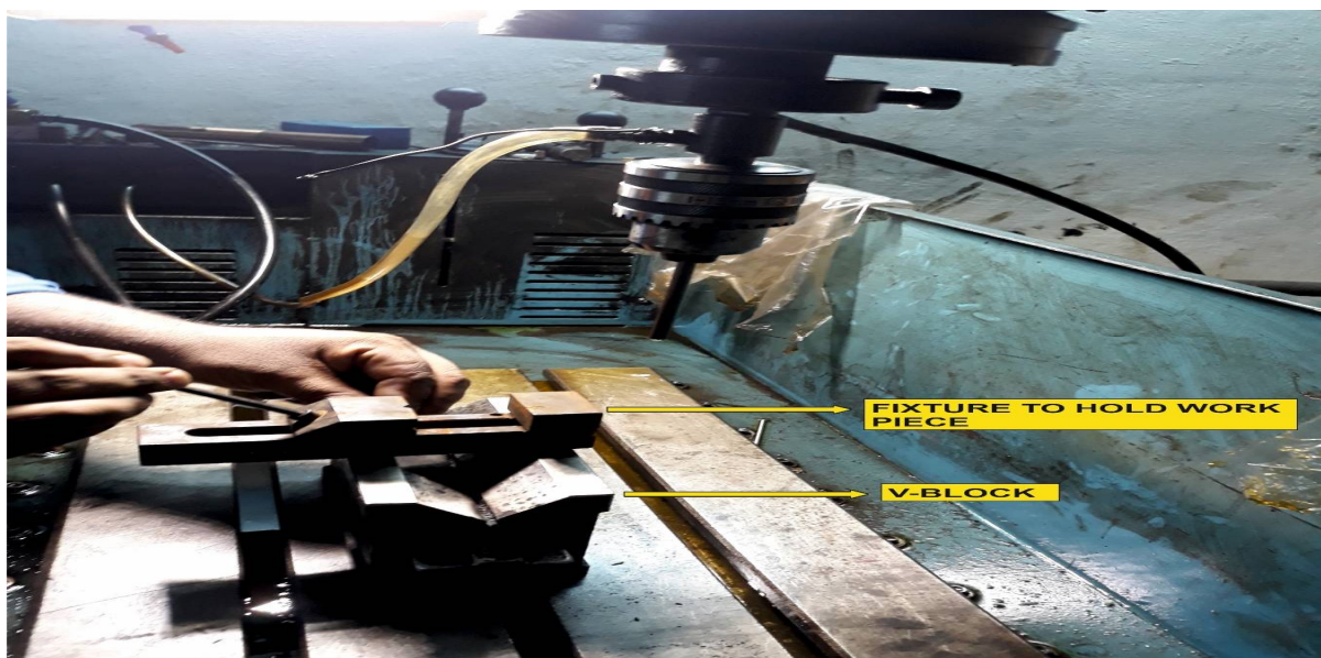
Fig. 3.2D work piece fixture arrangement
