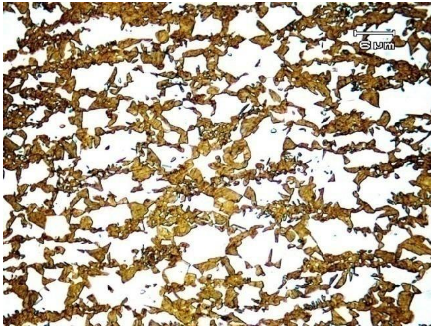
Figure 1.1 microstructure of steel “ferrite-martensite”
