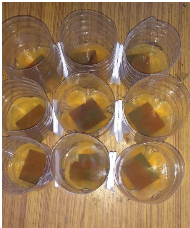
Figure 3.7 Samples after 15 days dipped in 5% NaCl solution
