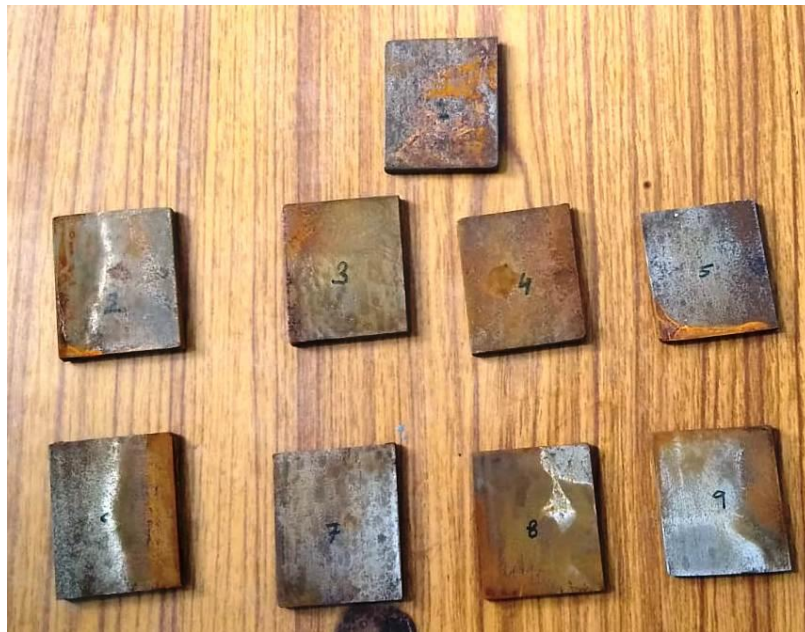
Figure 3.8 Samples condition after corrosion test
