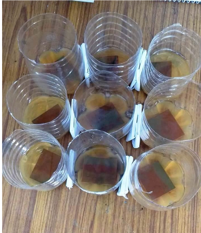
Figure 3.6 Samples dipped in 5% NaCl solution for the corrosion experiment
