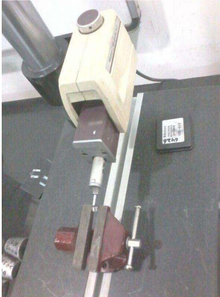
Figure4.6 Mitutoyo 178-602 Surface Roughness Tester Measuring. The Roughness Of Surface Machined By Wire-Edm
