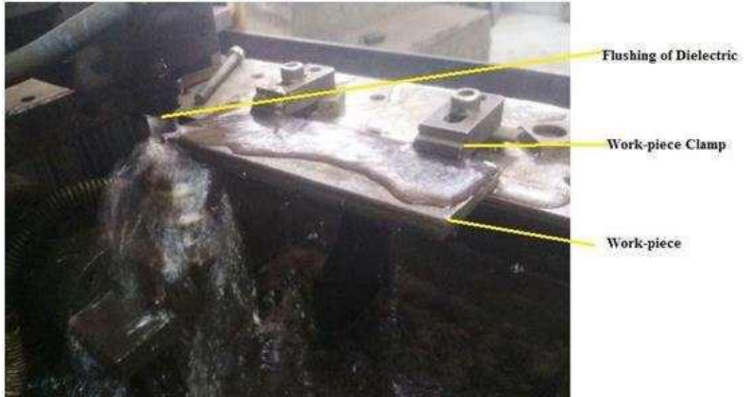
Figure 4.2 Machining on Electronica Wire-EDM
