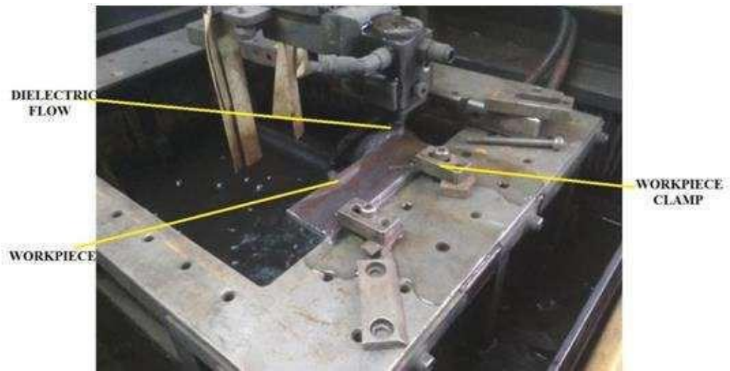
Figure 4.3 Parts of Electronica Wire-EDM
