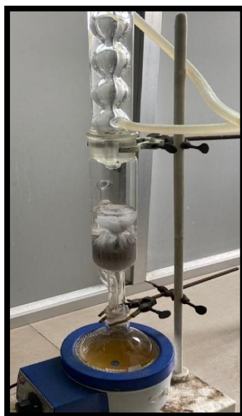
Fig. 3: Preparation of Cydonia oblonga Mill. extract using Soxhlet apparatus.
