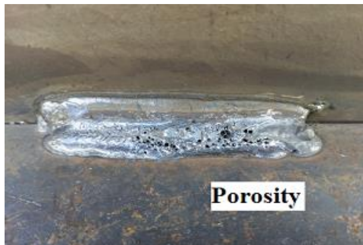
Figure 2.3 Porosity in Welding
