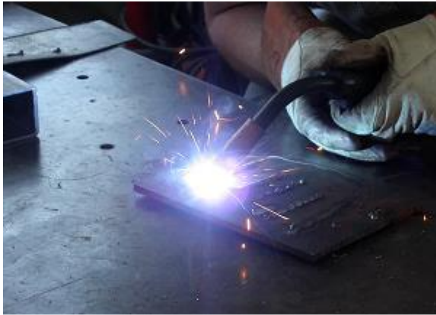
Figure 5.2 Surface Welding of Specimen
