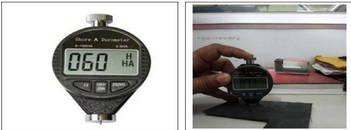
Figure 3.11 Shore A hardness tester & testing of workpiece
