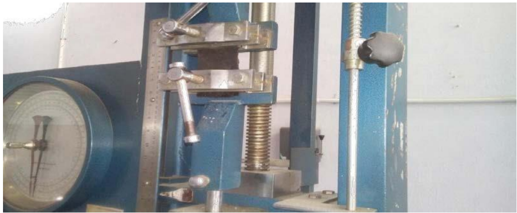
Figure 3.9 Tensile testing machine (work piece is ready for tensile test)
