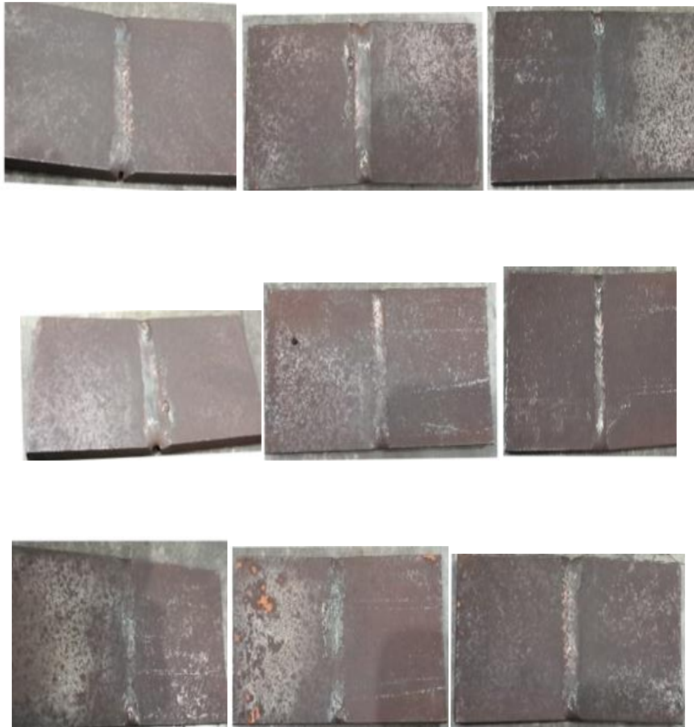
Fig. 11 Welded specimens performed with 3 different speed and current setting by conventional autogenous TIG welding process
