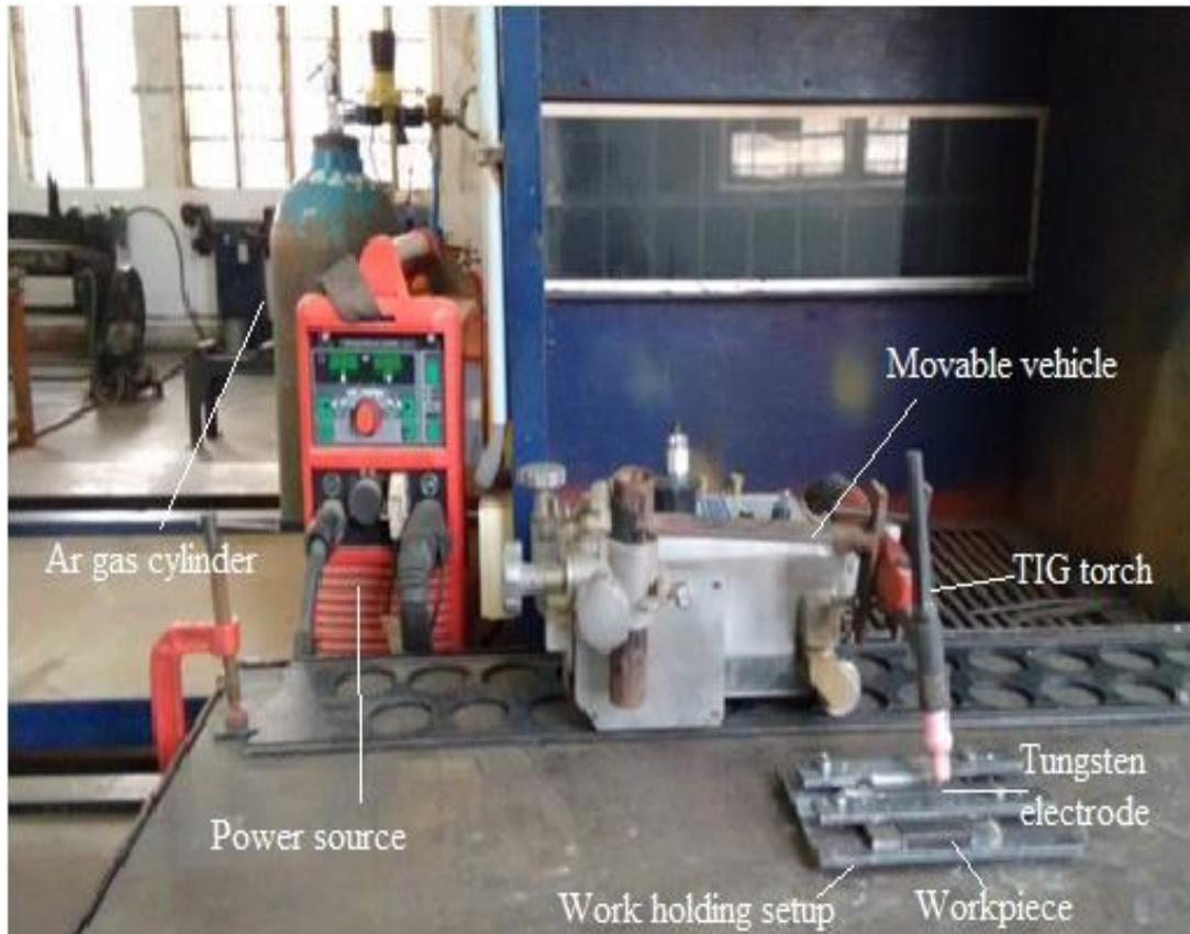
Fig. 3 Experimental setup of TIG welding
