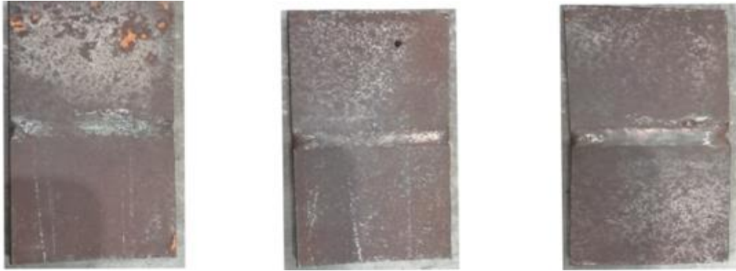
Fig. 15 TIG welded specimen with TiO 2 flux at 250 A current
