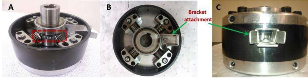
Figure 35: (A) Painted outside race; (B) Custom bracket attachment utilized in test rig setup; and (C) Camera view during measurements.
