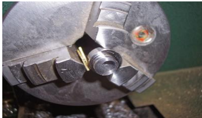
Fig 7: Eccentric Turning (Ref-www.google.com)
