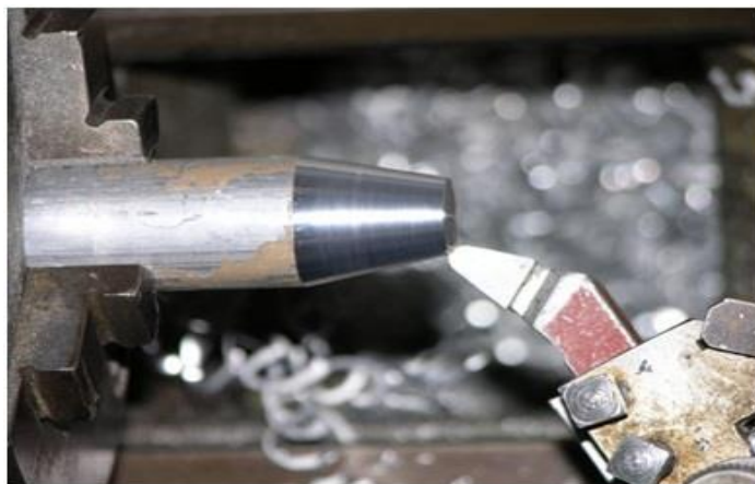
Fig 4: Taper Turning (Ref-www.google.com)
