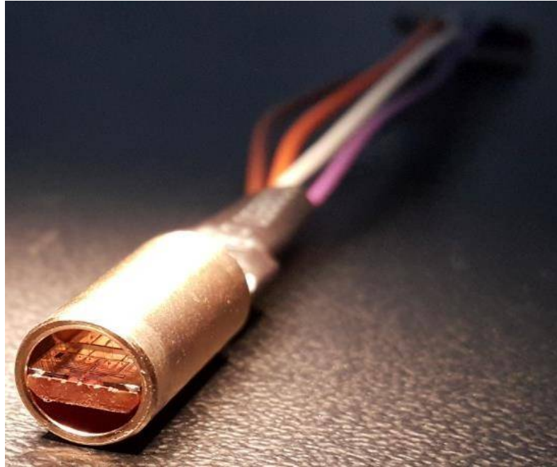
Figure 7.10 - Close up view of a sensor inside the cylinder with its electrical connections completed.
