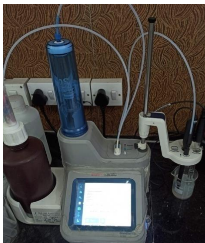
FIGURE3.3.7a: Chloride by Auto titrator
