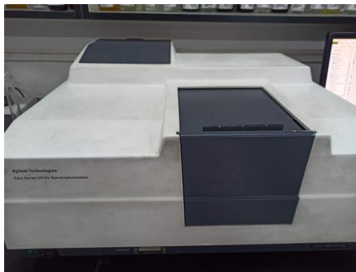
FIGURE3.3.10.1b: Sulphate detection by Spectrophotometer.
