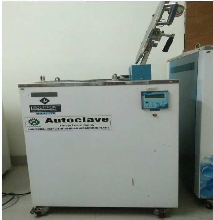
Figure 9-Vertical autoclave for sterilization of spawn substrate
