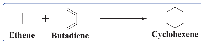
Fig. (1). Diels Alder reaction showing 100% atom efficiency.
