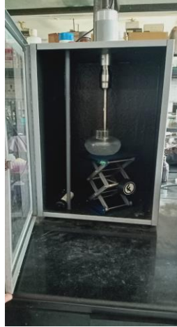
Figure6: An instrument used for ultra-sonication process during nanoemulsion synthesis
