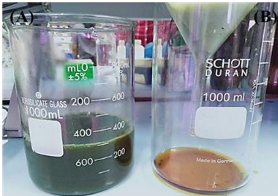
Figure 3 (a) Beaker (on left hand) showing filtered plant extract with the muslin cloth (b) Beaker (on right hand) showing filtered plant extract with 20 \mu\text{m} Whatman filter paper.
