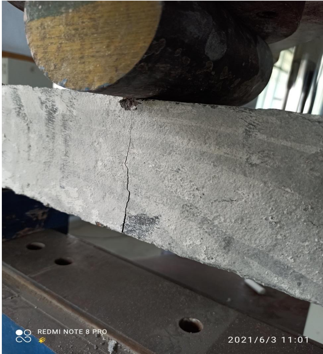
Fig3.3.6 Flexural strength testing
