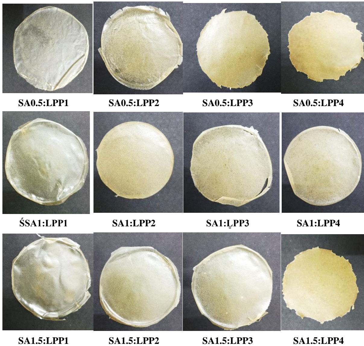
Figure 3.10. Developed biodegradable films using sodium alginate and lemon peel.
