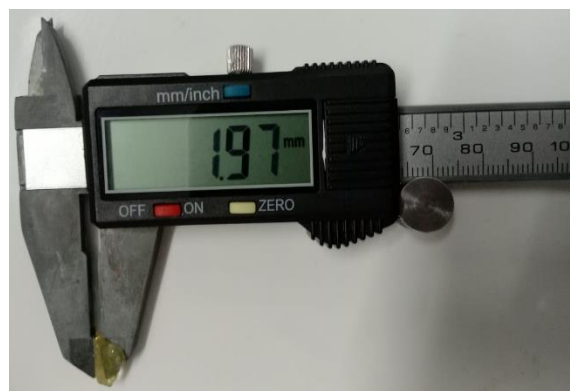
Plate 25 Measurement of membrane thickness
