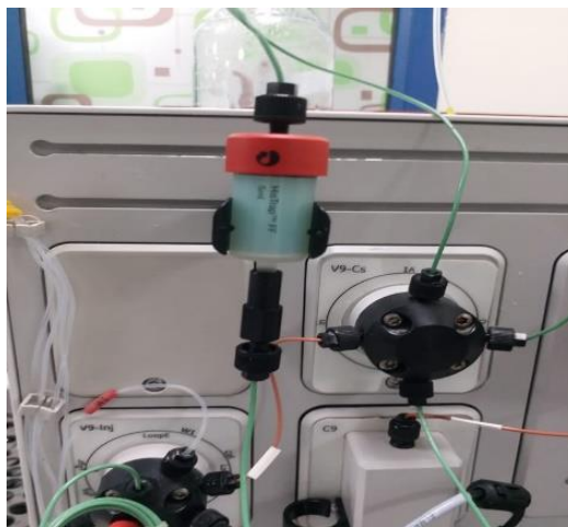
Fig.12. illustrates the utilization of a 5ml prepaccked Ni-NTA column for purifying a His-tagged protein.
