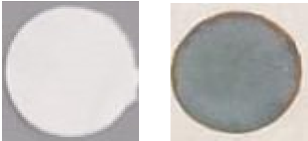
Figure 18. (a) The assay design: the device was incorporated with proline (10 \mu l of concentration 1 mg/ml) at the four reservoirs after being fabricated (grey region represents the hydrophilic area of the device); (b) isatin solution was introduced from central inlet zone; it penetrated into each detection zone and triggered different colour changes (pyrrole blue colour). The arrow in figure b shows the increasing amino acid content.
