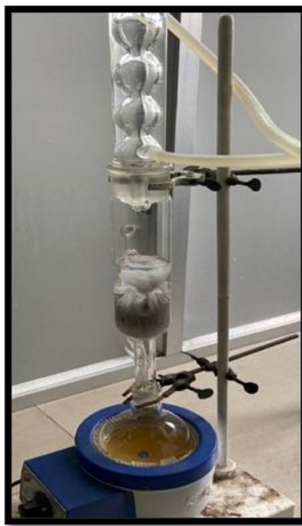
Figure 2. Preparation of Cydonia oblonga Mill. extract using Soxhlet apparatus.
